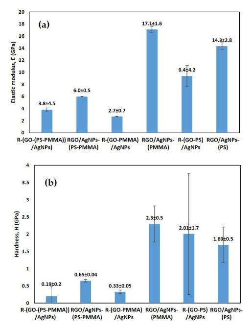
Figure 9. Berkovich nanoindentation: (a) elastic modulus and (b) hardness.
