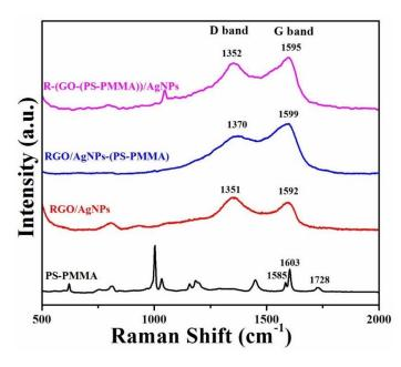
Figure 4. Raman spectra of PS-PMMA, RGO/AgNPs, RGO/AgNPs-(PS-PMMA), and R-(GO-(PS-PMMA)-AgNPs.
