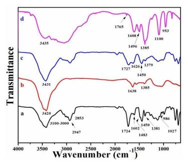
**Figure 1.** FT-IR spectra of (**a**) polystyrene (PS)-polymethylmethacrylate (PMMA), (**b**) reduced graphene oxide (RGO)/silver nanoparticles (AgNPs), (**c**) RGO/AgNPs-(PS-PMMA), and (**d**) R-(GO-(PS-PMMA)-AgNPs.
