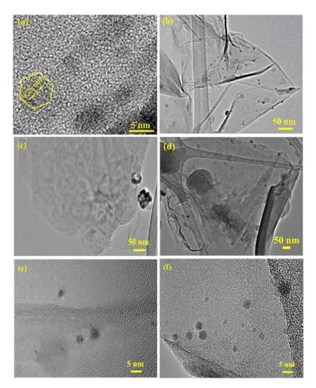
**Figure 6.** HR-TEM images of (**a**) AgNPs, (**b**) RGO/AgNPs, (**c**,**e**) RGO/AgNPs-(PS-PMMA), and (**d**,**f**) R-(GO-(PS-PMMA)-AgNPs.
