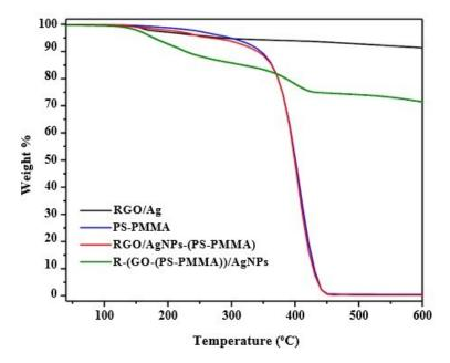
Figure 7. TGA thermograms for RGO/AgNPs/PS-PMMA nanocomposites.
