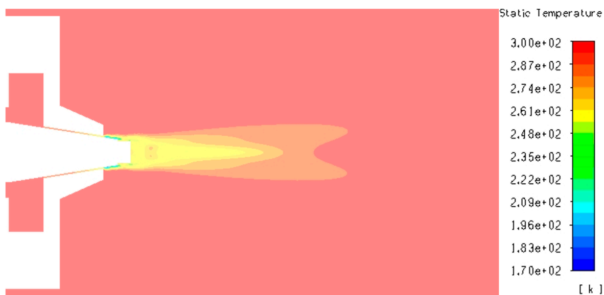
Figure S47. Temperature contour of k- \epsilon turbulent flow through SBS nozzle at 4 bar.
