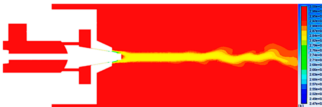
Figure S12. Temperature contour of laminar flow through SBS nozzle at 2 bar after 5000 iterations.
