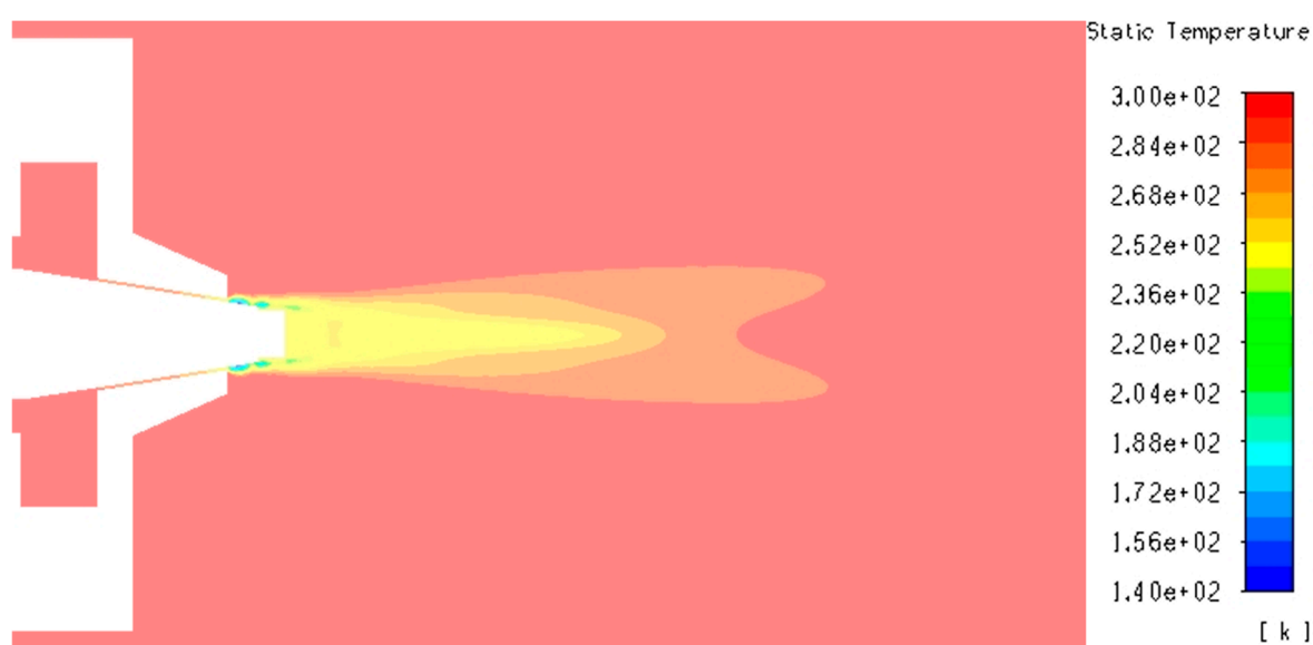
Figure S61. Temperature contour of k-ε turbulent flow through SBS nozzle at 6 bar.
