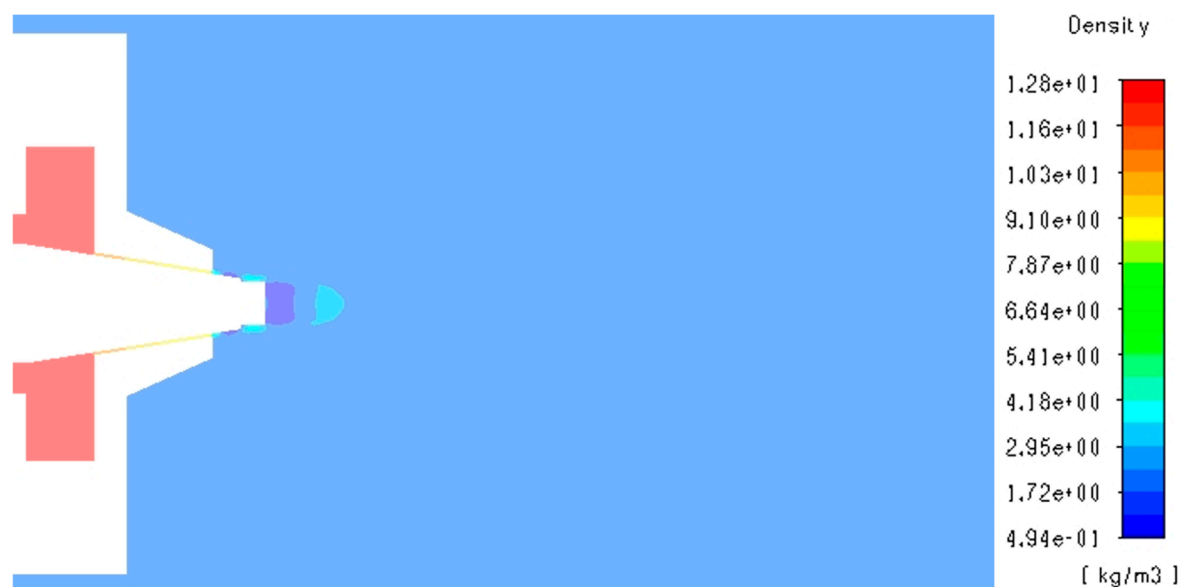
Figure S71. Density contour of k-ε turbulent flow through SBS nozzle at 10 bar.
