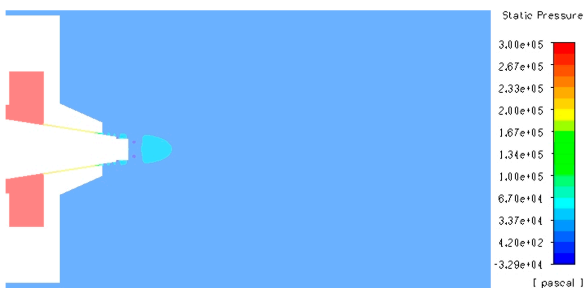
Figure S39. Pressure contour of k-ε turbulent flow through SBS nozzle at 3 bar.
