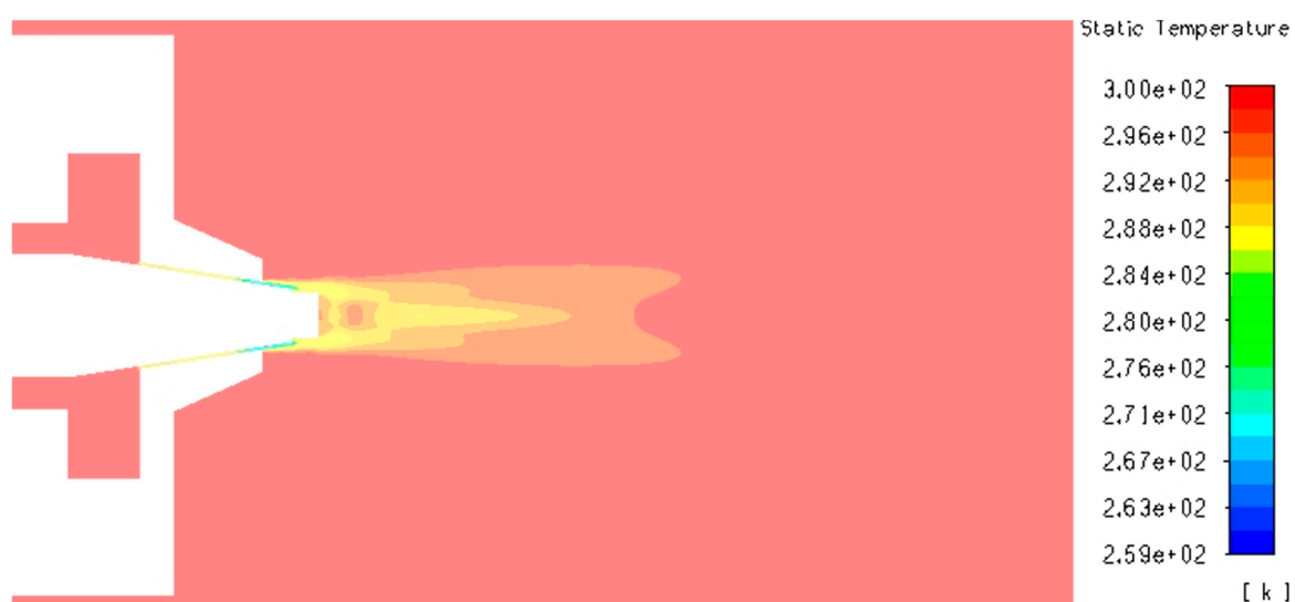
Figure S26. Temperature contour of k- \epsilon turbulent flow through SBS nozzle at 1 bar.
