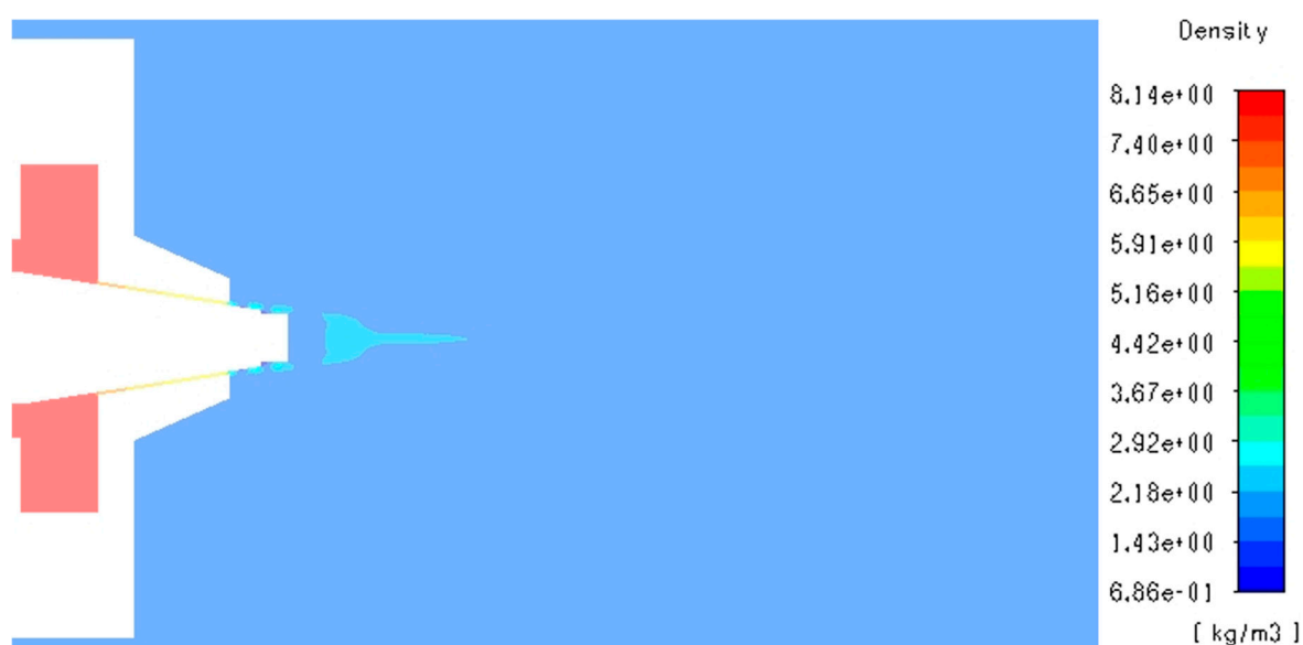
Figure S64. Density contour of k- \epsilon turbulent flow through SBS nozzle at 6 bar.
