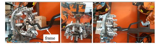
**Figure 22.** Test 2—Frame passage testing through fiber-processing head for calculated optimal REE trajectory.
