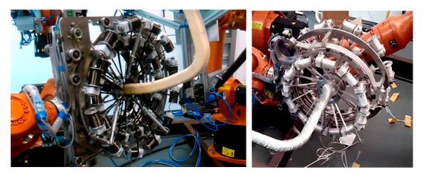
**Figure 6.** Different views of robot KR 16-2 with non-bearing core frame and fiber-processing head with three guide lines.
