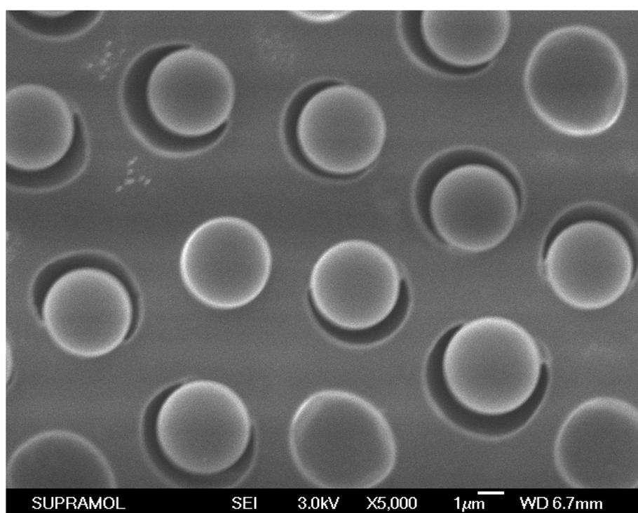
**Figure S1.** SEM images of porous films filled of PS microspheres with the content 0.1% w/v after washing with water.
