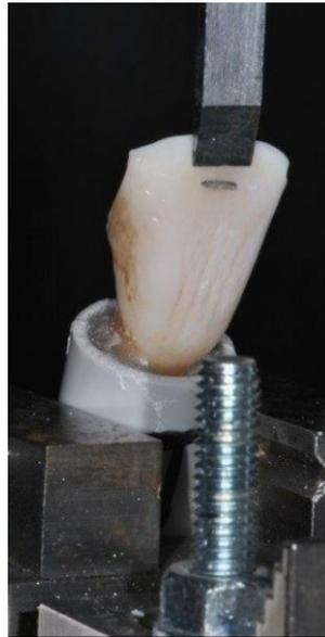
**Figure 3.** Positioning of specimens into the universal testing machine (three-quarter view).
