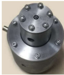
(b) The assembled gas-assisted extrusion die
