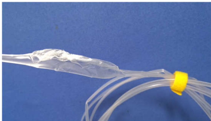
Figure 2. Polypropylene (PP) micro-tube with swelling and fracture.
