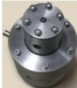
(b) The assembled gas-assisted extrusion die
