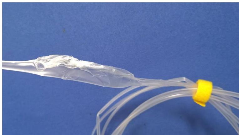
**Figure 2.** Polypropylene (PP) micro-tube with swelling and fracture.
