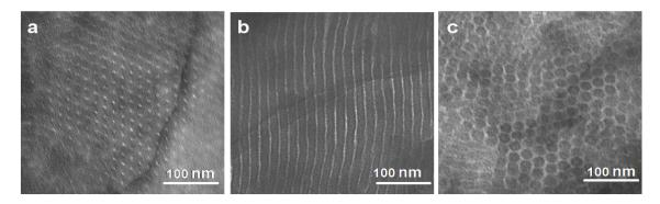
**Figure 4.** Transmission electron microscopy (TEM) micrographs of S-*b*-F block copolymers: (**a**) S74-*b*-F7, (**b**) S74-*b*-F17, and (**c**) S74-*b*-F42.
