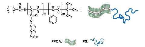
**Scheme 1.** Chemical structure of poly(styrene-*block*-perfluorooctylethyl acrylate) block polymers and corresponding illustration.
