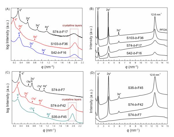
**Figure 2.** Small-angle X-ray scattering (SAXS) curves of S-*b*-F samples showing (**A**) lamellar and (**C**) hexagonal morphology. Layered crystalline PFOA structures could be identified in wide-angle region (**B**,**D**).
