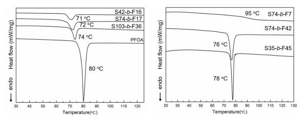
**Figure 1.** Differential scanning calorimetry (DSC) curves of S-*b*-F block polymer and perfluorooctylethyl acrylate (PFOA) homopolymer.
