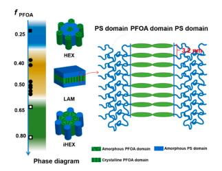
**Figure 5.** Phase diagram and illustration of hierarchical structure of S-*b*-F block copolymers. Solid square, solid sphere, and hollow square represent experiment data for hexagonally packed cylinders (HEX), lamellar layers (LAM), and inverse hexagonally packed cylinders (iHEX) phases.
