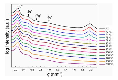
Figure 3. Temperature-dependent SAXS profiles of S74-b-F42.
