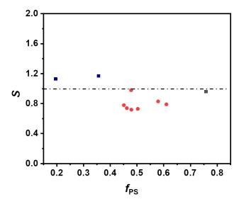
**Figure 6.** Plot of stretching ratios for polystyrene chains (*S*) versus  $f_{PS}$  for all S-*b*-F samples. Black square, HEX; red dot, LAM; and blue square, iHEX.
