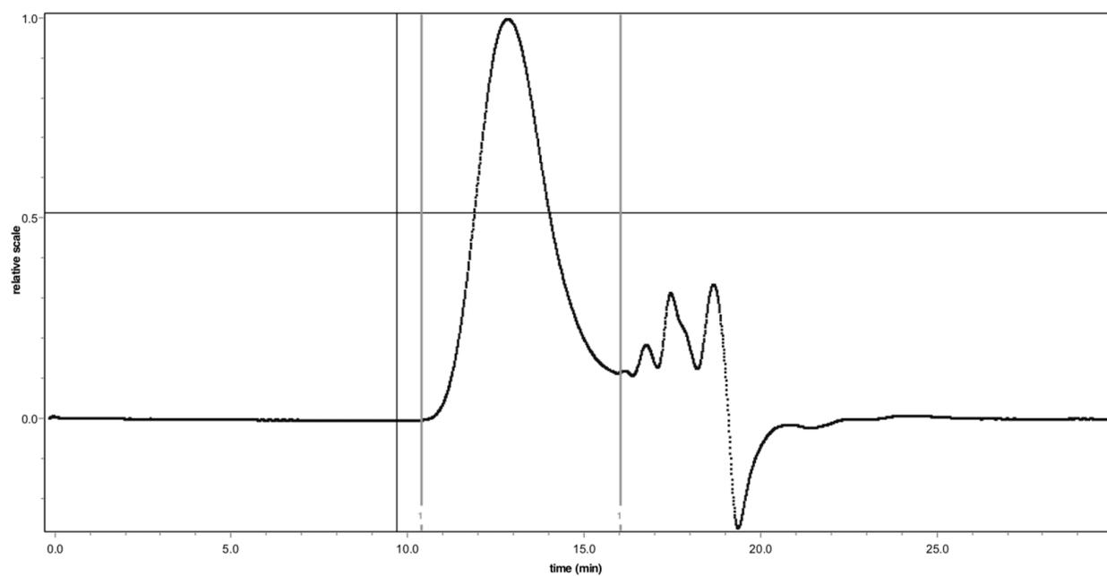
**Figure S2.** SEC trace (DMF eluent containing 10 mM LiBr, refractive index detection) for PBSe ( $M_n = 30$  kg/mol and  $D = 1.9$ ).
