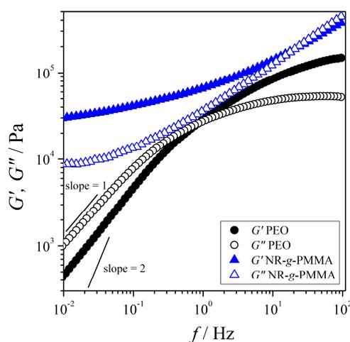
**Figure 1.** The variation of  $G'$  (solid markers) and  $G''$  (open markers) with frequency at  $T = 140 \text{ °C}$ . The results for PEO are indicated by circles; the results for NR-g-PMMA are indicated by triangles.
