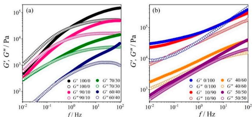
**Figure 3.** Plots of storage modulus (closed marker) and loss modulus (open marker) as a function of frequency for PEO/NR-g-PMMA at  $T = 140\text{ }^{\circ}\text{C}$ : (a) blends with the excess PEO content and (b) blends with the excess NR-g-PMMA content.
