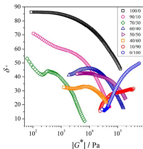
**Figure 7.** Van Gorp-Palmen plots of PEO/NR-g-PMMA blends at  $T = 140^\circ\text{C}$ .
