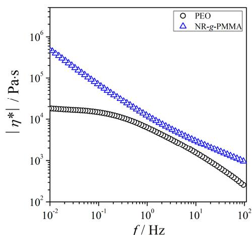
**Figure 2.** Plots of complex viscosity as a function of frequency for PEO and NR-g-PMMA at  $T = 140\text{ }^{\circ}\text{C}$ . The results for PEO are indicated by circles; the results for NR-g-PMMA are indicated by triangles.
