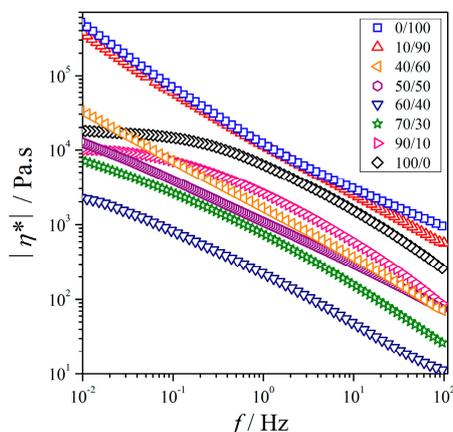
**Figure 5.** Complex viscosity versus frequency for PEO/NR-g-PMMA blends at  $T = 140^\circ\text{C}$ .
