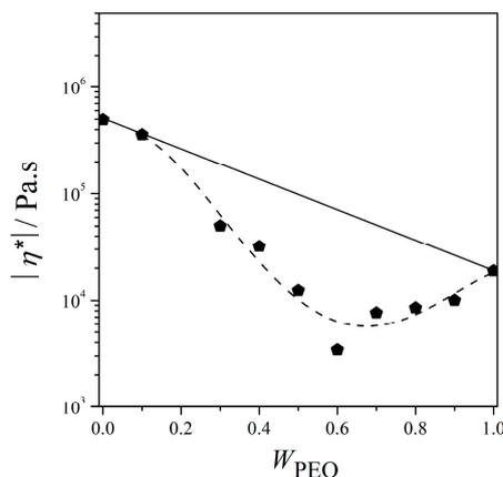
**Figure 6.** Viscosity evaluated at  $f = 0.01$  Hz as a function of mass fraction of PEO at  $T = 140$  °C. The solid curve represents the additive curve as in Equation (7). The dashed curve is the 4th polynomial regression curve with  $R^2 > 0.95$  for visual inspection (*cf.* text).
