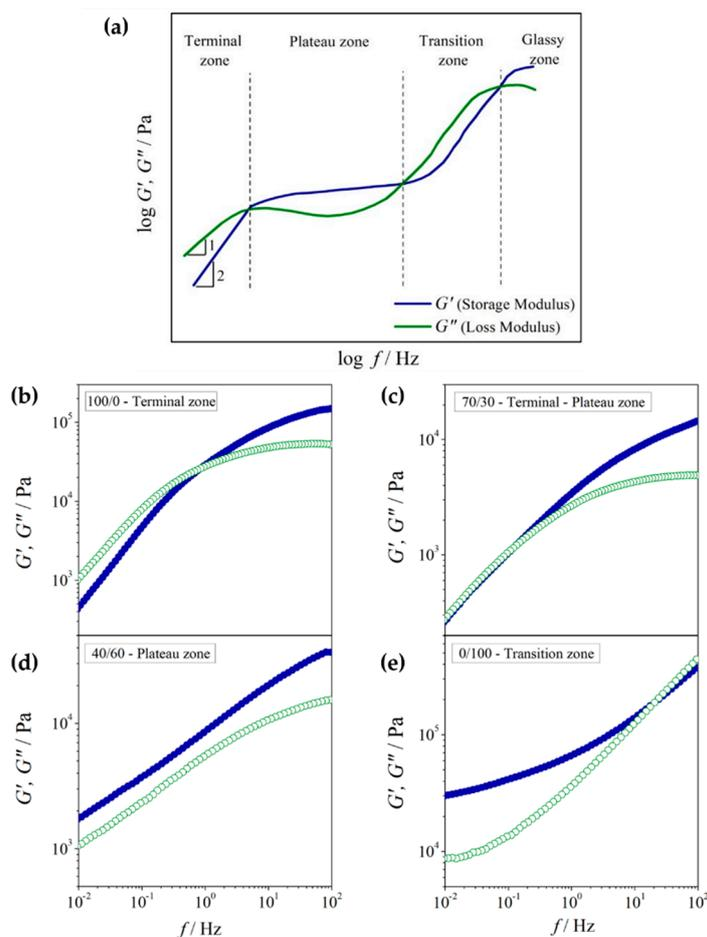
**Figure 4.** Plots of  $G'$  and  $G''$  as a function of frequency for (a) three-zone model and PEO/NR-g-PMMA blends of (b) 100/0 (c) 70/30 (d) 40/60 and (e) 0/100.
