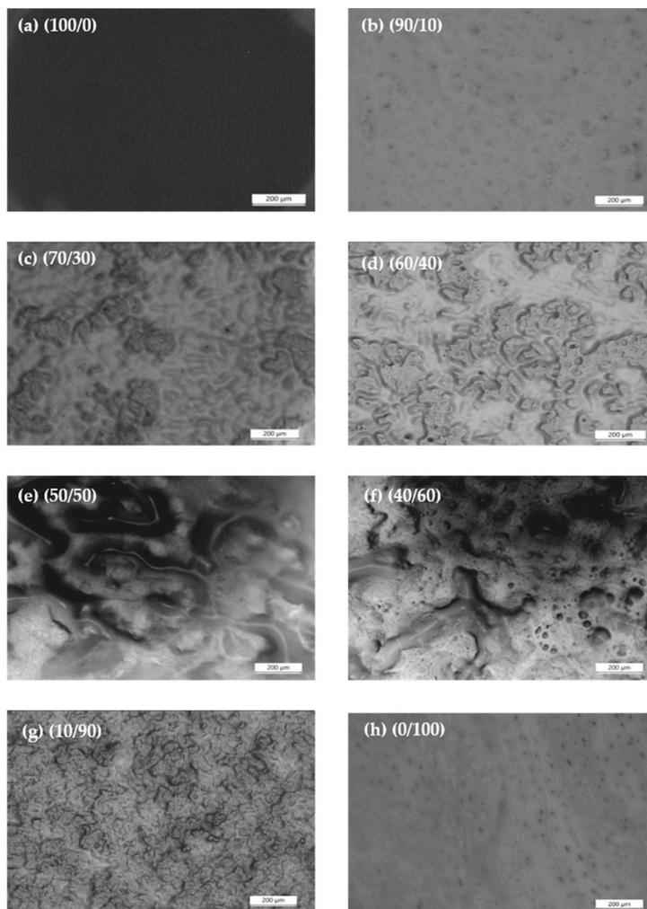
**Figure 8.** Optical microscopy images of PEO/NR-g-PMMA for (a) 100/0 (b) 90/10 (c) 70/30 (d) 60/40 (e) 50/50 (f) 40/60 (g) 10/90 and (h) 0/100 blends captured at  $T = 140\text{ }^{\circ}\text{C}$  after 10 min.
