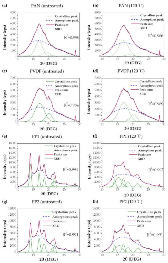
Figure S3. XRD patterns of untreated and heat treated filter sebs.
