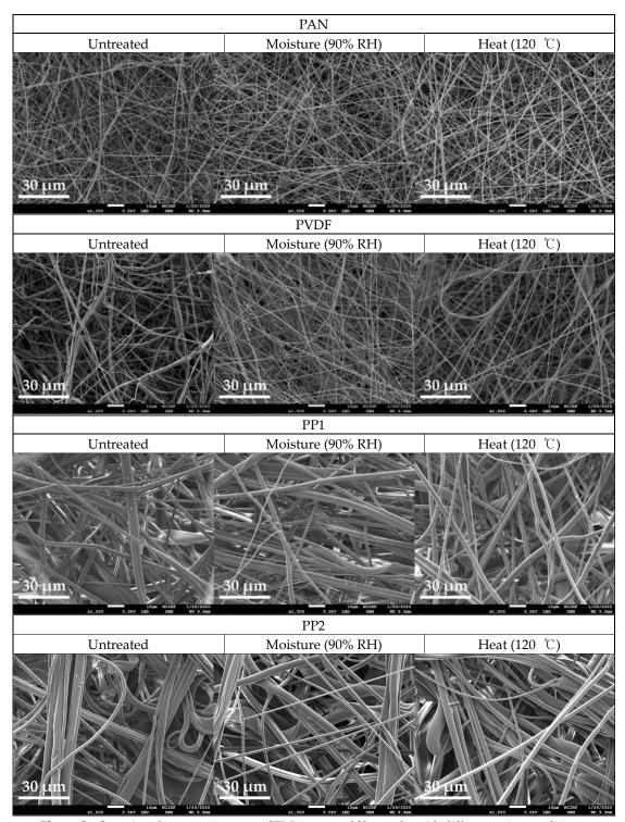
Figure S1. Scanning electron microscope (SEM) images of filter webs with different aging conditions.
