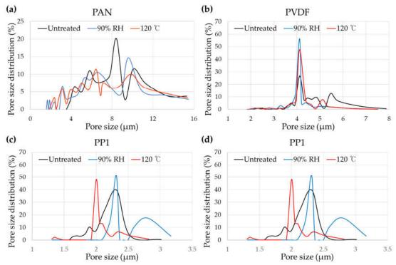
Figure S2. Pore size distribution of filter webs.
