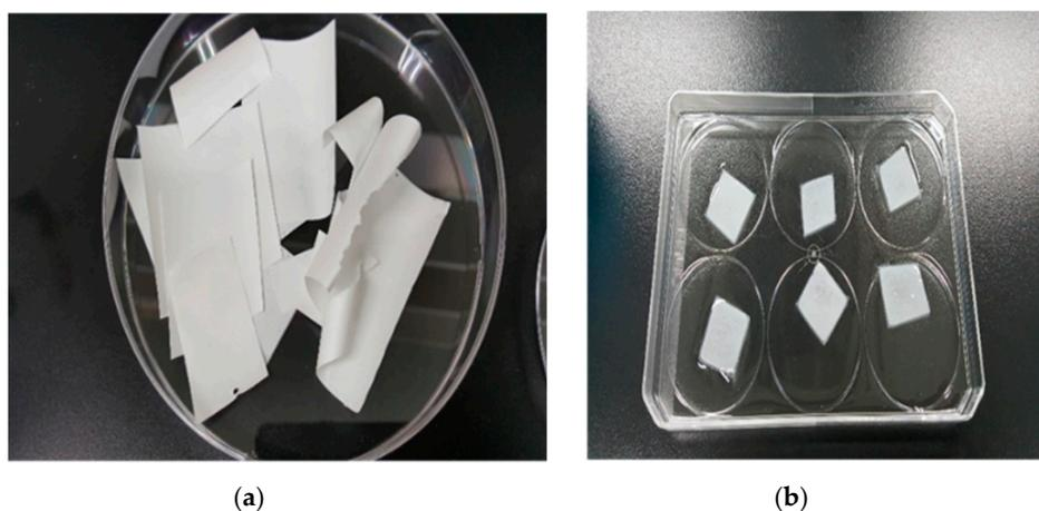
**Figure 1.** (a) is an alginate/carboxymethyl cellulose (CMC)/polyethylene oxide (PEO) nanofiber film obtained from the collector after electrospinning. (b) shows the alginate/CMC/PEO nanofiber film during the crosslinking process with CaCl<sub>2</sub> solution.
