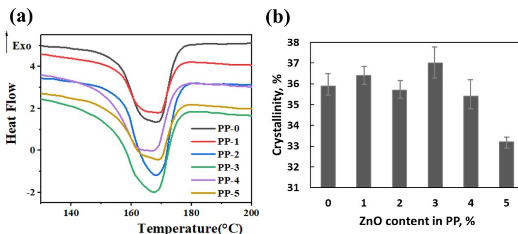
Figure 6. (a) Differential scanning calorimetry (DSC) heating curves and (b) crystallinities of PP fibers.
