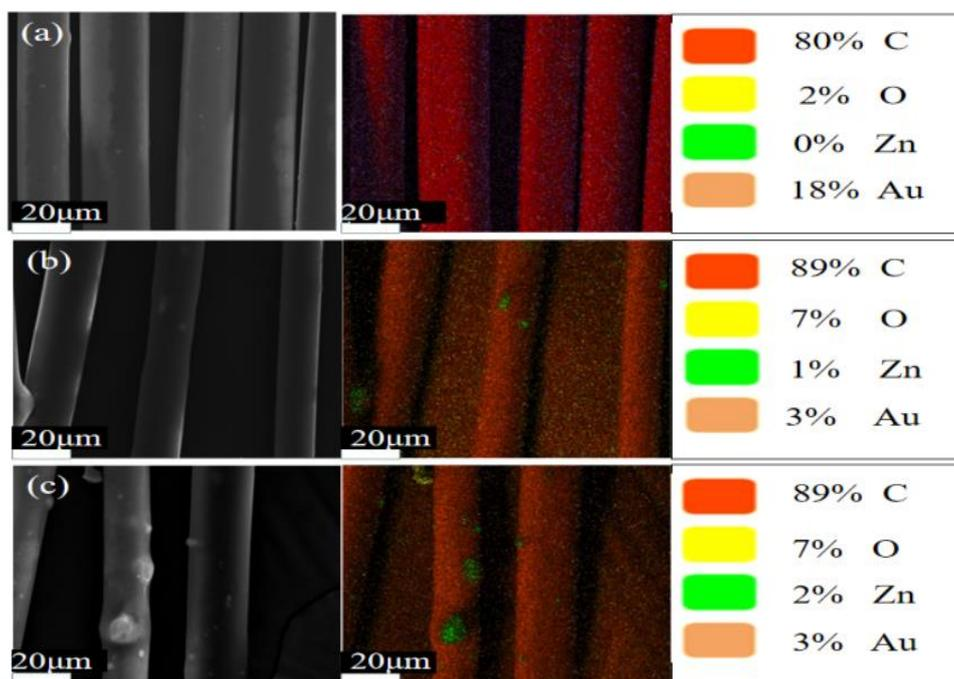
Figure 4. SEM/energy-dispersive spectroscopy (EDS) patterns of PP e-spun fibers containing ZnO: (a) 0 wt.%; (b) 1 wt.%; (c) 3 wt.%.
