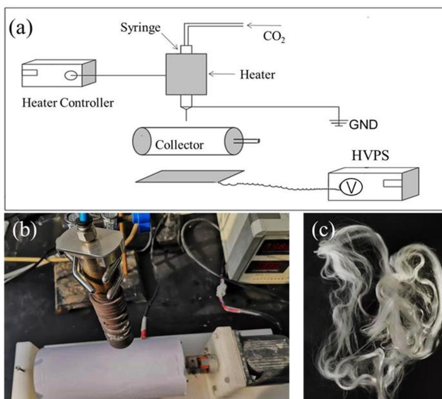
**Figure 1.** (a) Home-made melt e-spinning device; (b) heating device; (c) melt e-spun polypropylene (PP) fibers.
