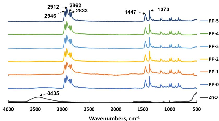
Figure 5. Fourier-transform infrared (FTIR) spectra of ZnO and e-spun PP fibers with different content of ZnO.
