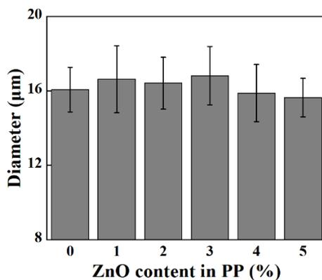
**Figure 3.** Average diameter of e-spun PP fibers.
