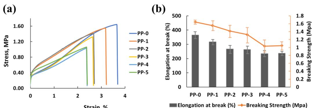
**Figure 8.** (a) Stress–strain behavior, and (b) trend of elongation at break and breaking strength of e-spun PP fibers.
