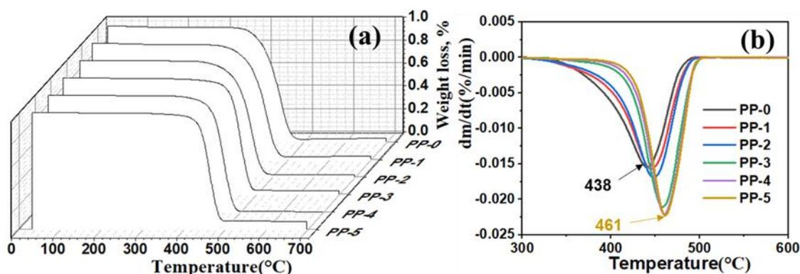
Figure 7. (a) Thermogravimetry (TG) traces of as-spun fibers and (b) differential TG (DTG) spectra.
