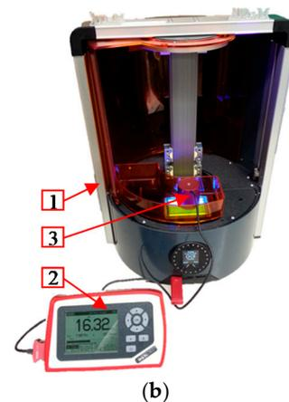
**Figure 4.** (a) A projected image with nine  $10 \times 10$  mm<sup>2</sup> squares having 155 grayscale pixel value, (b) measuring the irradiance of the Ember machine using a power meter.
