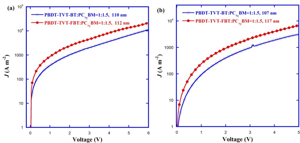
**Fig. S7** *J-V* curves of hole-only (a) and electron-only (b) devices for the PBDT-TVT-BT:PC<sub>71</sub>BM and PBDT-TVT-FBT:PC<sub>71</sub>BM.
