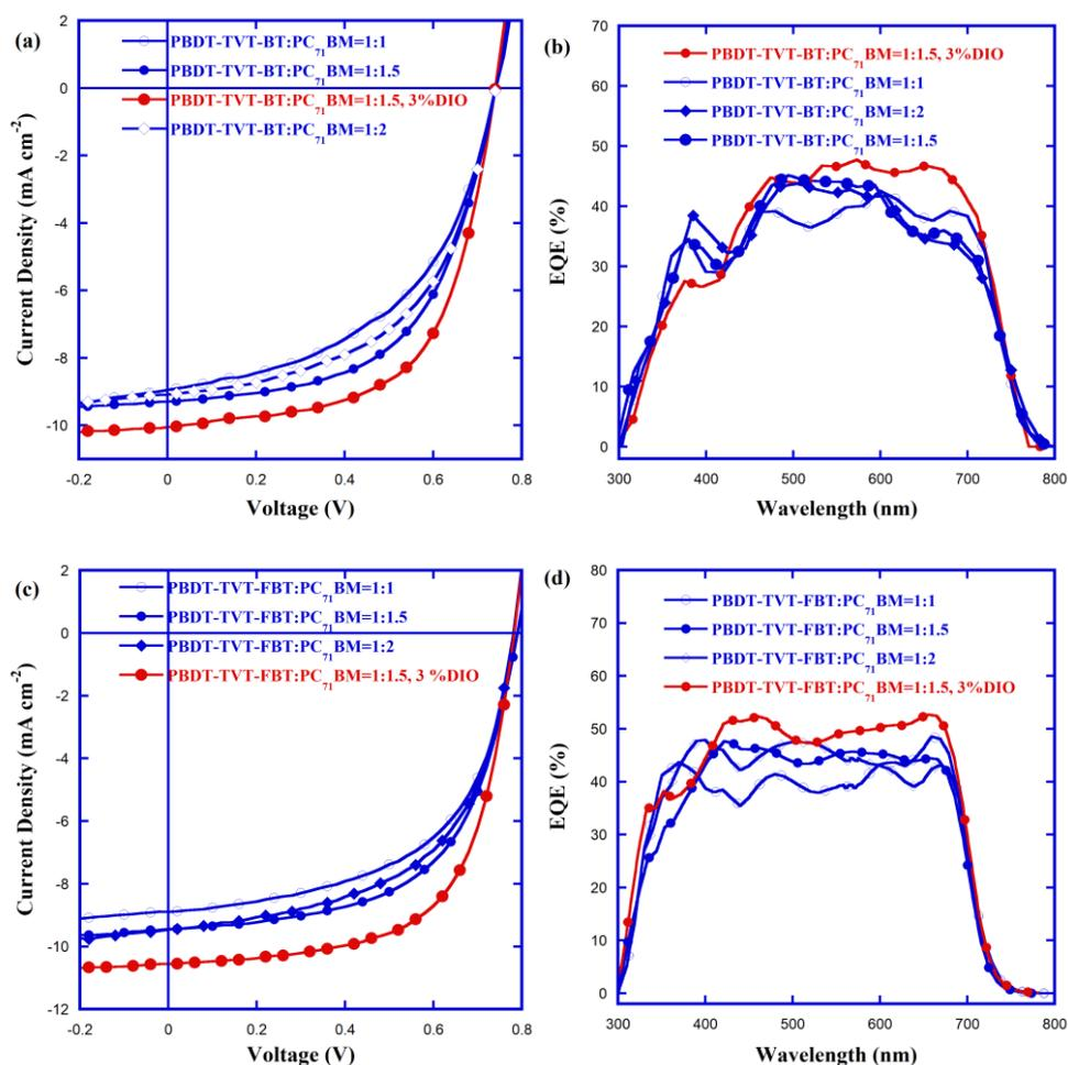
**Fig. S6** *J-V* curves of PBDT-TVT-BT and PBDT-TVT-FBT with different weight ratio to PC<sub>71</sub>BM, and using 3%DIO additive and EQE spectra of corresponding PSCs.
