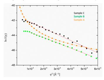
**Figure 8.** Guinier extrapolation of the ZnO radius for sample C (black) and B (green). Sample A (orange) clearly shows a deviation from the Guinier dependence.
