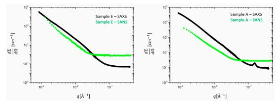
**Figure 1.** Absolutely calibrated SAXS (black) and SANS (green) data for samples E (left) and A (right). The data are not background-corrected.
