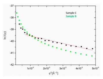
**Figure 7.** Guinier extrapolation for the silica cluster radius for sample C (black). The fit cannot be uniquely applied to sample B (green) due to the strong deviation from linearity.
