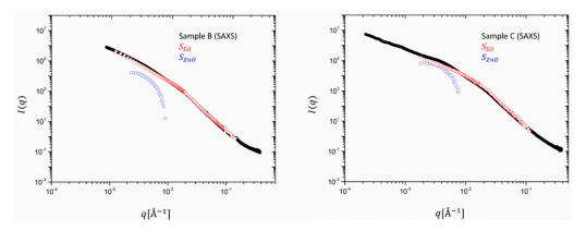
**Figure 4.** Experimental SAXS data in absolute intensity units cm<sup>-1</sup> for samples B (30 phr) (left) and C (60 phr) (right). Partial form factors for silica ( $S_{pol}$ , red) and ZnO ( $S_{ZnO}$ , blue) were multiplied by the contrast factors to re-construct the intensity.
