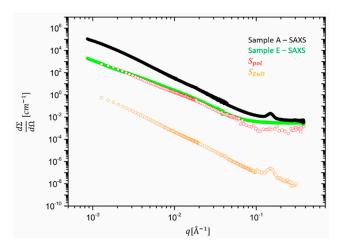
**Figure 2.** Partial structure factors  $S_{pol}$  (red) and  $S_{ZnO}$  (orange) as derived from sample A in comparison with absolutely calibrated SAXS data for samples A (black) and E (green).  $S_{pol}$  was arbitrarily shifted to be compared with sample E.
