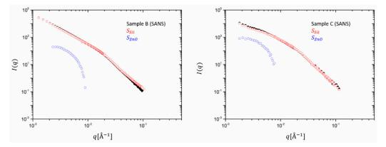
**Figure 5.** Experimental SANS data in absolute intensity units cm<sup>-1</sup> for samples B (30 phr) (left) and C (60 phr) (right). Partial form factors for silica ( $S_{pol}$ , red) and ZnO ( $S_{ZnO}$ , blue).
