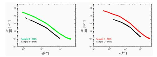
**Figure 3.** Experimental SANS and SAXS data in absolute intensity units cm<sup>-1</sup> for the ZnO-containing filled rubbers, sample B (left) and sample C(right). The number of data points of the ultrahigh-resolution SAXS data was about 4500 and was reduced to a SANS-compatible lower resolution of about 350 data points by means of a cubic spline fitting procedure.
