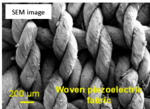
**Figure 5.** SEM image shows the microstructure of a woven piezoelectric fabric obtained using the plied yarns. Reprinted with permission from Enlong Yang, Zhe Xu, Lucas K. Chur, Ali Behroozfar, Mahmoud Baniyadi, Salvador Moreno, Jiacheng Huang, Jules Gilligan, Majid Minary-Jolandan, Nanofibrous smart fabrics from twisted yarns of electrospun piezopolymer, *ACS Applied Materials and Interfaces* 2017, Vol. 9, 24220–24229. Copyright (2017), American Chemical Society.
