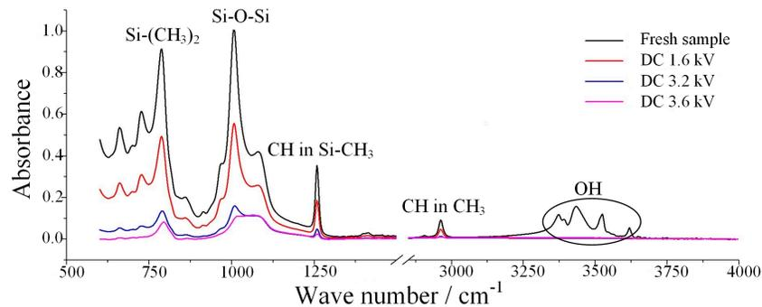
**Figure 11.** FTIR spectra at different applied voltages ( $\gamma_{20} = 1000 \mu\text{S}/\text{cm}$ ,  $t = 8 \text{ h}$ )**Table 8.** The absorption peak height of bands in the FTIR spectrum.
