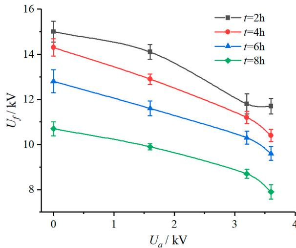
**Figure 6.** Relationship between *U<sub>f</sub>* and *U<sub>a</sub>* ( $\gamma_{20} = 3000 \mu\text{S/cm}$ ).
