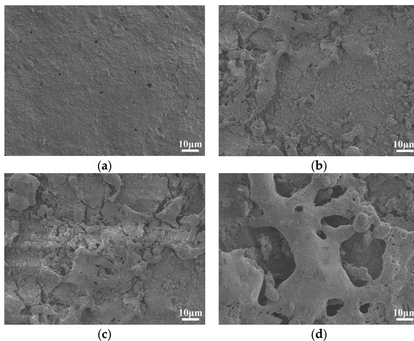
**Figure 10.** SEM images at different applied voltage ( $\gamma_{20} = 1000 \mu\text{S}/\text{cm}$ ,  $t = 8 \text{ h}$ , 1000 $\times$ ). (a) DC 0 kV, (b) DC 1.6 kV, (c) DC 3.2 kV, (d) DC 3.6 kV.
