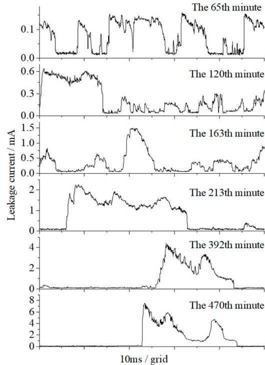
**Figure 5.** The typical waveform of leakage current (DC 3.2 kV,  $\gamma_{20} = 5000 \mu\text{S/cm}$ ).
