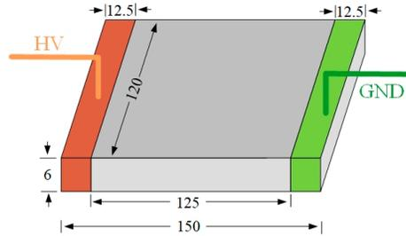
Figure 1. Tested samples (unit: mm).
