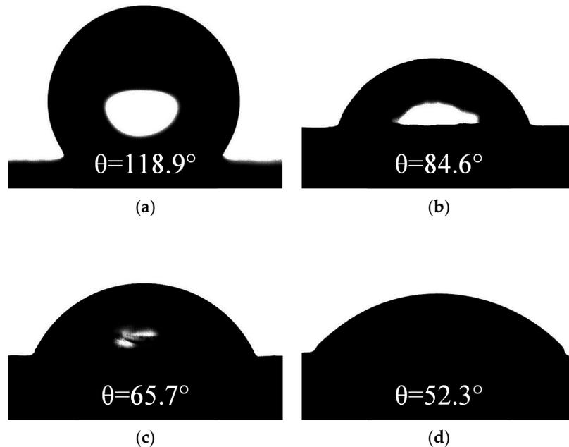
**Figure 9.** Static contact angles at different applied voltages ( $\gamma_{20} = 1000 \mu\text{S}/\text{cm}$ ,  $t = 8 \text{ h}$ ). (a) DC 0 kV, (b) DC 1.6 kV, (c) DC 3.2 kV, (d) DC 3.6 kV.
