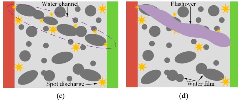
**Figure 8.** Development of flashover of HTV SR sample in salt-fog environment. (a) Water drops deposit, (b) water drops deformation, (c) partial discharge, (d) flashover.
