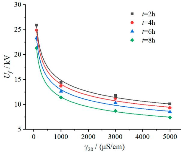
Figure 3. Relationship between  $U_f$  and  $\gamma_{20}$  (DC 3.2 kV).
