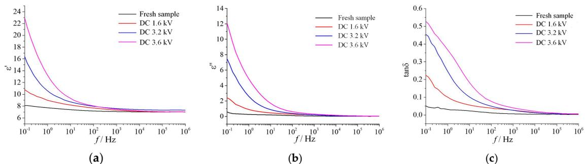
**Figure 12.** The dielectric parameters at different applied voltage ( $\gamma_{20} = 1000 \mu\text{S}/\text{cm}$ ,  $t = 8 \text{ h}$ ). (a) Real part, (b) imaginary part, (c) dielectric loss factor.
