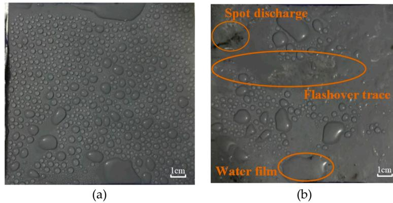
**Figure 7.** Surface states of the samples after salt-fog treatment. (a) Unenergized (0 kV), (b) energized (DC 3.2 kV).
