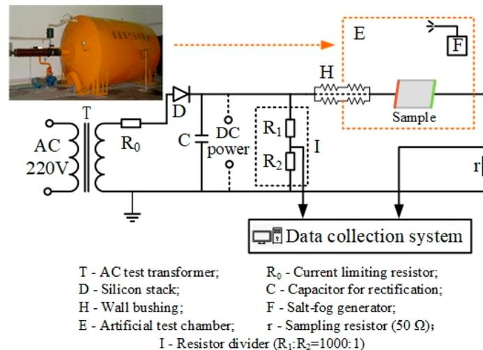
Figure 2. Schematic diagram of DC test circuit.
