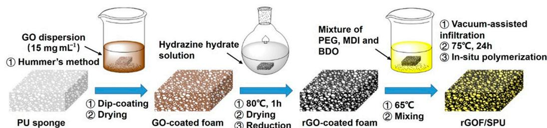
**Figure 1.** Schematic illustration of the synthetic route to preparing the reduced graphene oxide (rGO)-coated foam (rGOF)/segmented polyurethane (rGOF/SPU) composite. PU, polyurethane.
