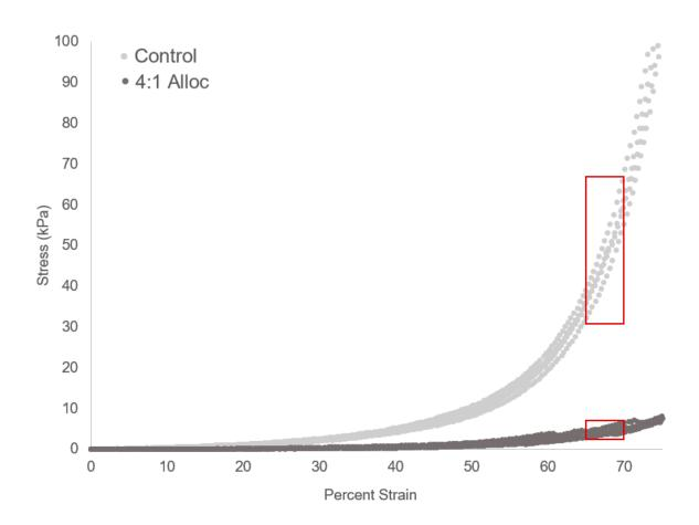
**Figure S1.** Stress-strain curves for PEGDA hydrogels. 0:1 (control) and 4:1 alloc to acrylate conditions. It can be seen that the hydrogels undergoing compression experience an elongated toe region before reaching the linear region. This linear region, corresponding to 65-70% strain, is outlined with a red box. The slope of this linear region was taken as the compressive modulus of each hydrogel.
