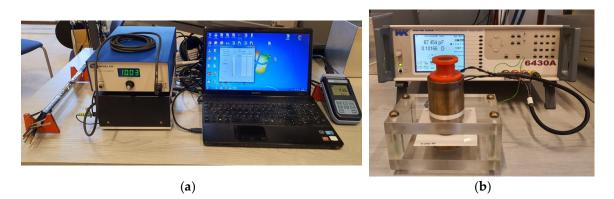
**Figure 5.** Measurement of dielectric properties: (**a**) voltage response measurement on a PVC cable sample; (**b**) measurement of PVC films by cylindrical copper electrodes by Wayne–Kerr 6430A impedance analyzer.
