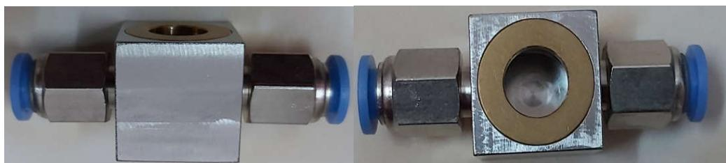
**Figure S3.** Stainless steel gas measuring cell
