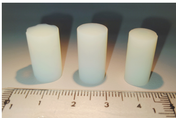
Figure S1. Image of CS/GPTMS-SiO 2 hybrid aerogel monoliths with different GPTMS content obtained by CO 2 supercritical drying. Left (CS4G0), centre (CS7G2) and right (CS10G4) samples containing 10.3, 8.0 and 9.7 wt. % chitosan, respectively
