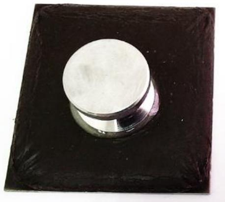
**Figure 2.** Dolly applied on the coating surface.
