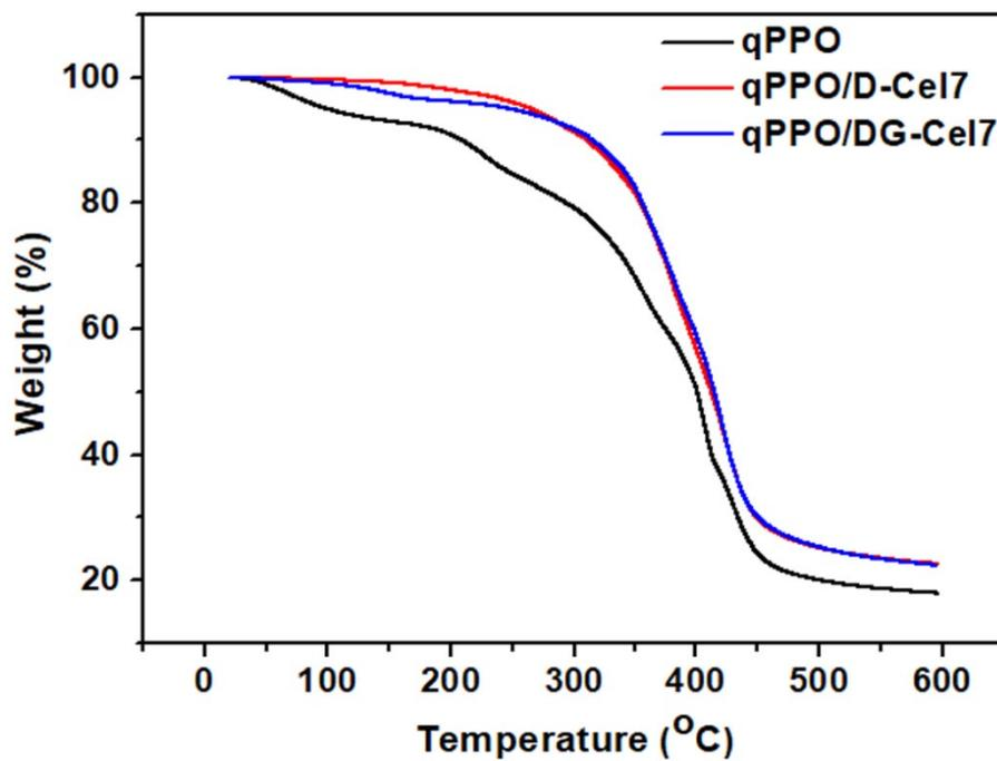
Figure S5. TGA graph of qPPO, qPPO/D-Cel7, and qPPO/DG-Cel7.
