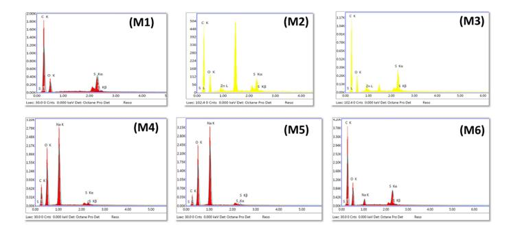
**Fig.S2** EDS point analysis of the electrospun co-axial nanofibers membranes before and after surface treatment.
