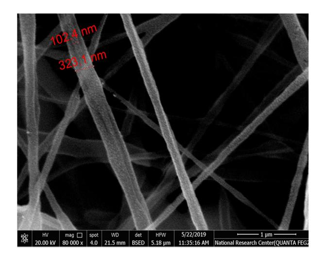
Fig.S1 high resolution image of coaxial nanofiber membrane.
