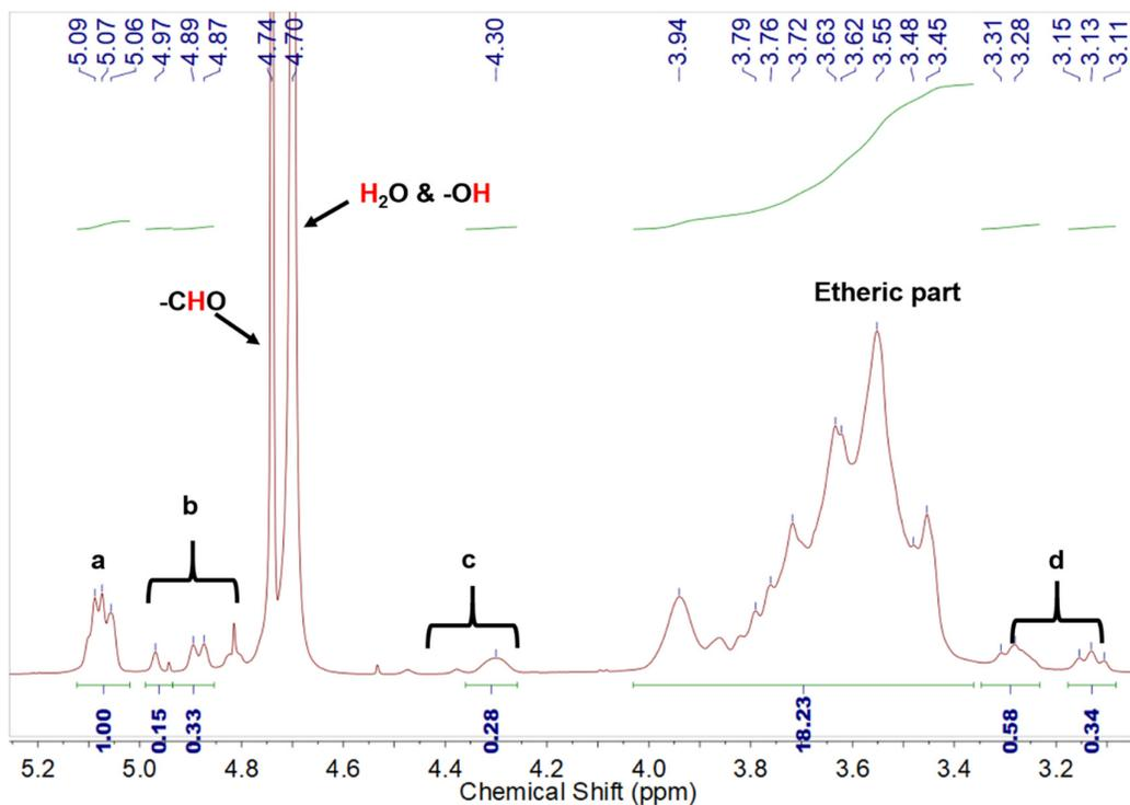
Figure S3. <sup>1</sup>H NMR spectrum and calculus information of aldehyde-terminated hbPGs (hbPGs reacted with 20 mg NaIO<sub>4</sub>) in D<sub>2</sub>O. The ratio between peak (5.08 ppm) and etheric skeleton is 18.23:1.
