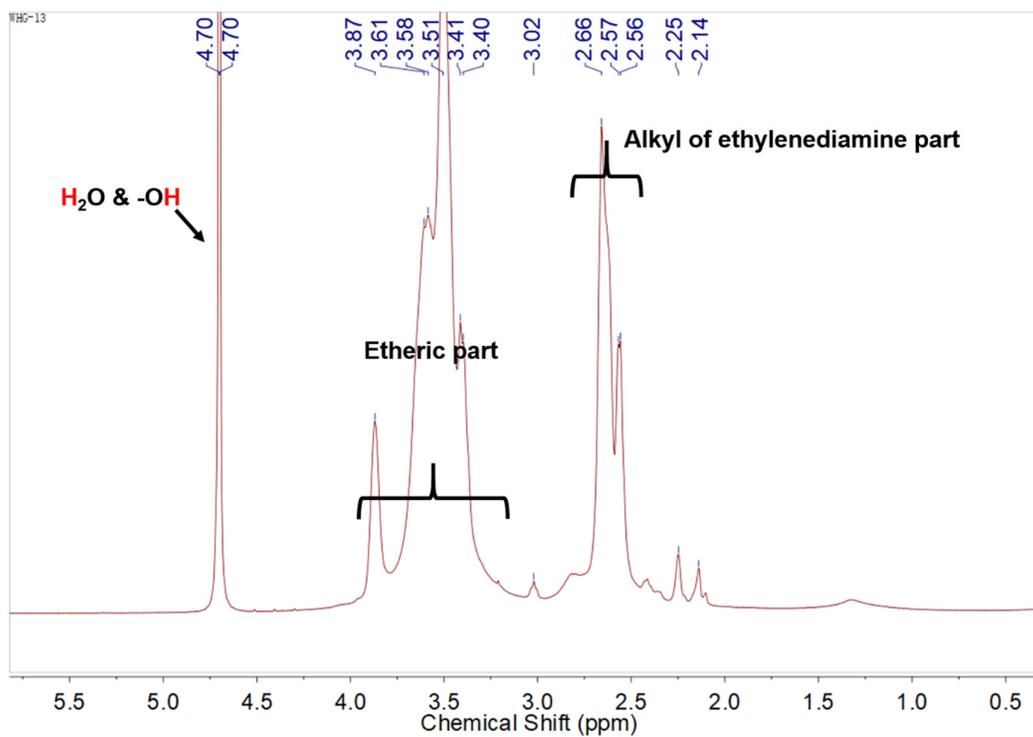
Figure S4.  $^1\text{H}$  NMR spectrum of hbPGs-NH<sub>2</sub> in D<sub>2</sub>O.
