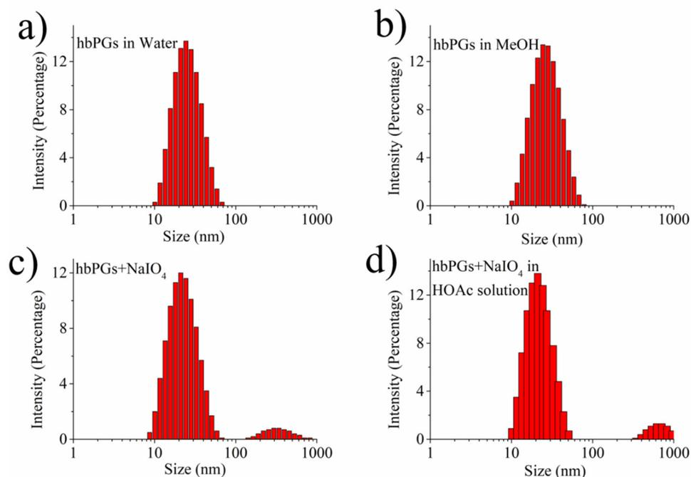
**Figure S6.** Hydrodynamic radius profile of (a) hbPGs in water, (b) hbPGs in MeOH, (c) hbPGs reacted with NaIO<sub>4</sub> (1.0 mg/mL) and (d) hbPGs reacted with NaIO<sub>4</sub> in HOAc solution (10% v/v aqueous solution).
