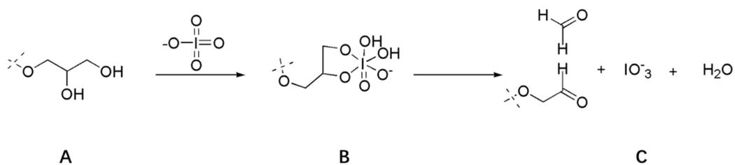
Figure 5. Reaction mechanism of vicinal diols oxidation using NaIO<sub>4</sub>. A-C are the step for NaIO<sub>4</sub> oxidation process: A, original reactant; B, addition products with NaIO<sub>4</sub>; C, final products.
