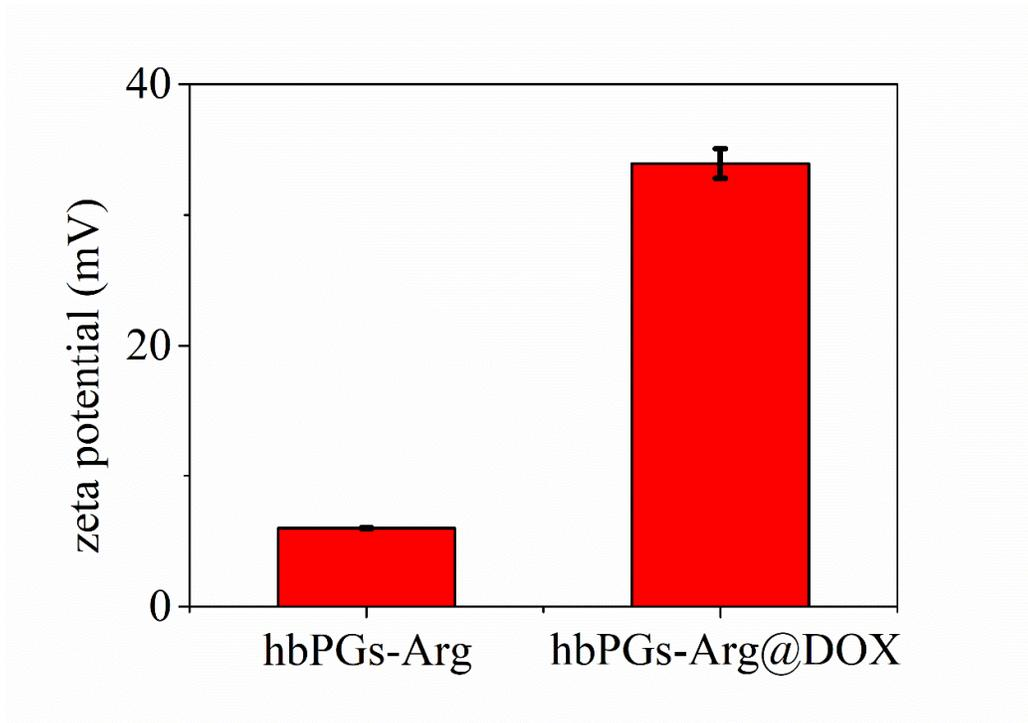
**Figure S9.** Zeta potential of hbPGs-Arg and hbPGs-Arg@DOX in aqueous solution (0.5 mg/mL for hbPGs-Arg).
