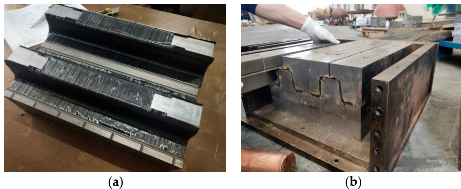
Figure 7. CFRP laminates on the molds and the closed molds: (a) laying up the prepreg; (b) closing the molds.
