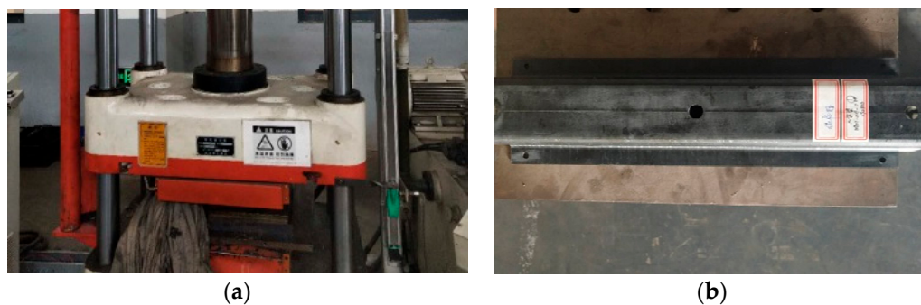
Figure 8. Heat-pressing forming of the prototype: (a) heating and pressing the structure; (b) the manufactured prototype.
