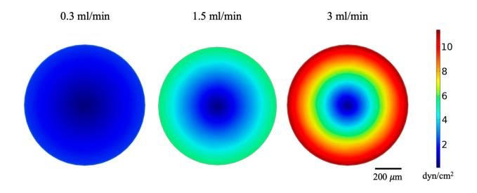
**Figure S1.** Simulated SS profiles across the channel at minimum (0.3 mL/min), medium (1.5 mL/min) and maximum flow rate (3 mL/min) imposed according to the theoretical analysis.
