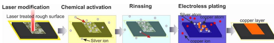
**Figure 1.** Steps of selective surface activation induced by laser (SSAIL) process: laser modification, chemical activation by dipping in the aqueous solution of silver nitrate, rinsing in distilled water and electroless copper deposition in the bath.
