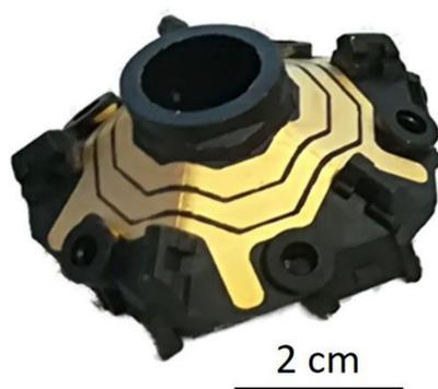
**Figure 16.** 3D MID item after SSAIL procedure, using pulse interlacing technique.
