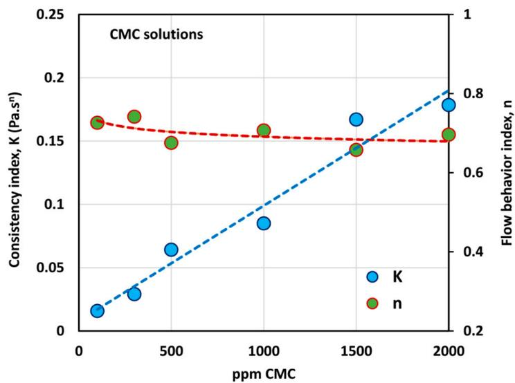
Figure 3. Variations of consistency index,  $K$ , and flow behavior index,  $n$ , with polymer (CMC) concentration.
