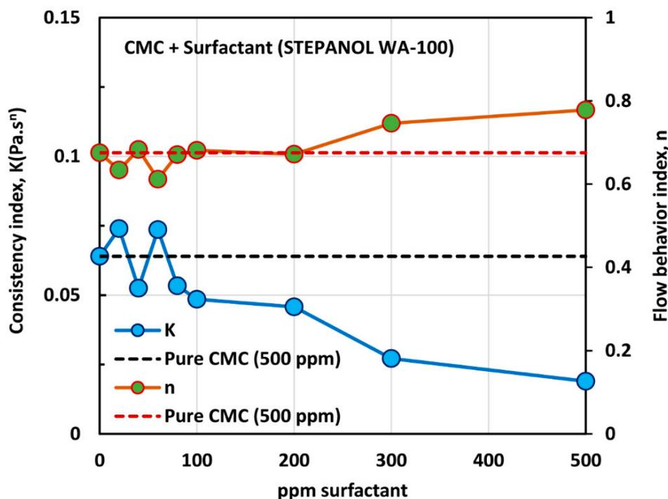
**Figure 9.** Variations of consistency index,  $K$ , and flow behavior index,  $n$ , for mixtures of anionic polymer CMC and anionic surfactant Stepanol WA-100 with the increase in surfactant concentration, at a fixed polymer concentration of 500 ppm.
