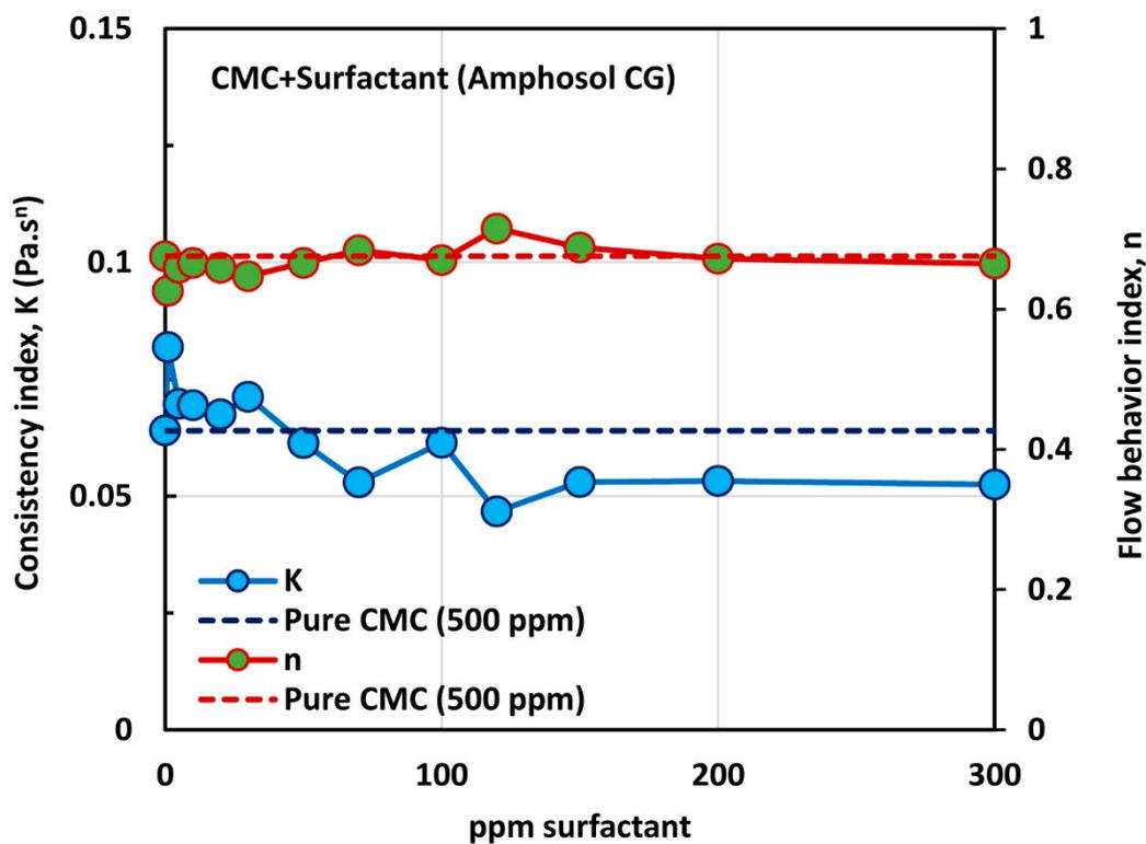
Figure 18. Variations of consistency index,  $K$ , and flow behavior index,  $n$ , for mixtures of anionic polymer, CMC, and zwitterionic surfactant, Amphosol CG, with the increase in surfactant concentration, at a fixed polymer concentration of 500 ppm.
