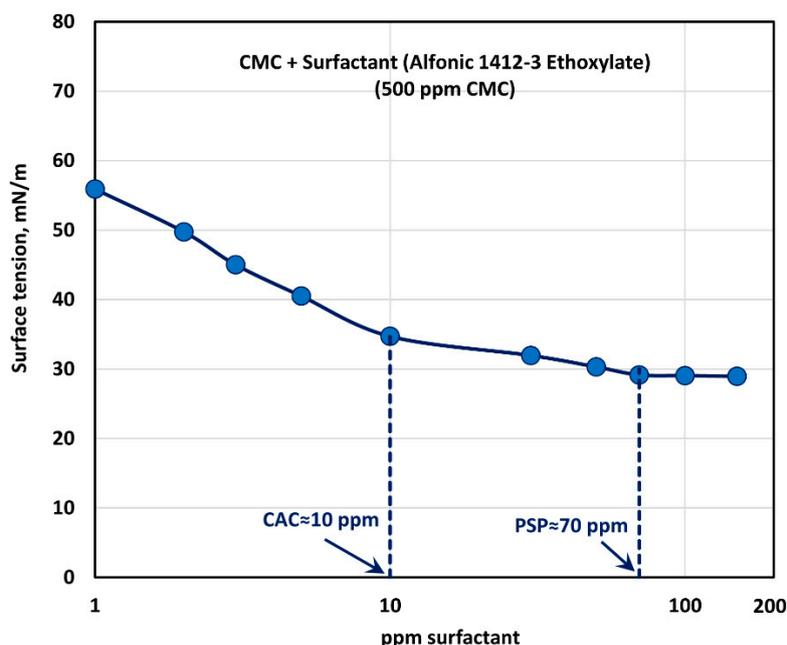
**Figure 13.** Variation of surface tension of surfactant-polymer solutions with the increase in surfactant (Alfonic 1412-3 Ethoxylate) concentration, at a fixed polymer (CMC) concentration of 500 ppm.
