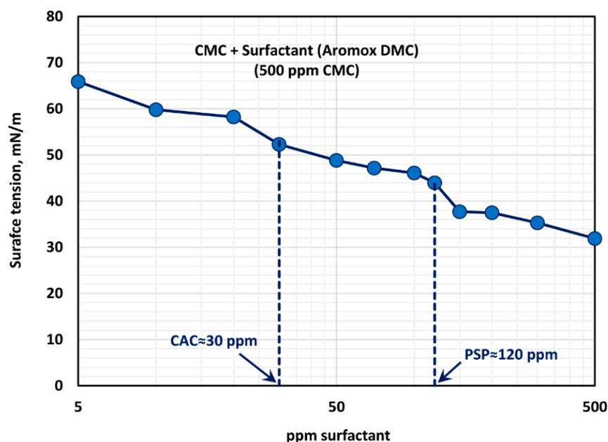
**Figure 16.** Variation of surface tension of surfactant-polymer solutions with the increase in surfactant (Aromox DMC) concentration, at a fixed polymer (CMC) concentration of 500 ppm.
