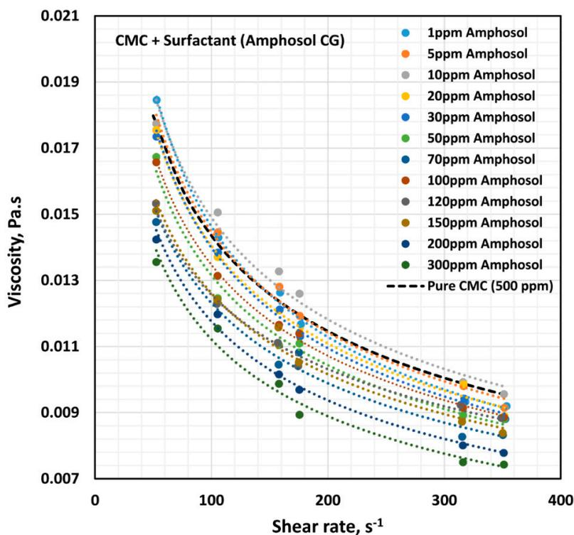
Figure 17. Effect of zwitterionic surfactant (Amphosol CG) on the viscosity versus shear rate behavior of solutions of mixtures of anionic polymer, CMC, and zwitterionic surfactant, Amphosol CG, at a fixed polymer concentration of 500 ppm.
