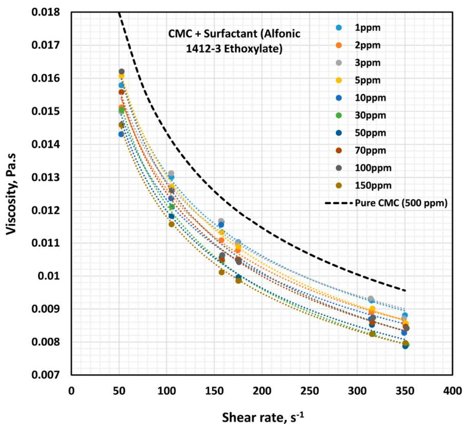
Figure 11. Effect of non-ionic surfactant (Alfonic 1412-3 Ethoxylate) on the viscosity versus shear rate behavior of solutions of mixtures of anionic polymer, CMC, and non-ionic surfactant, Alfonic 1412-3 Ethoxylate, at a fixed polymer concentration of 500 ppm.
