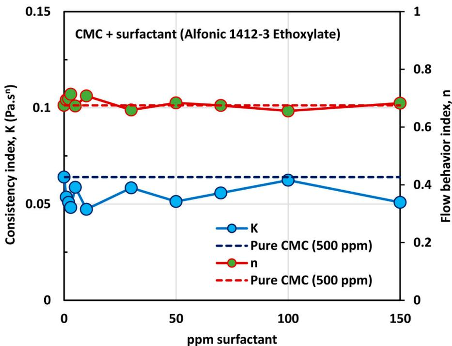
Figure 12. Variations of consistency index,  $K$ , and flow behavior index,  $n$ , for mixtures of anionic polymer, CMC, and non-ionic surfactant, Alfonic 1412-3 Ethoxylate, with the increase in surfactant concentration, at a fixed polymer concentration of 500 ppm.
