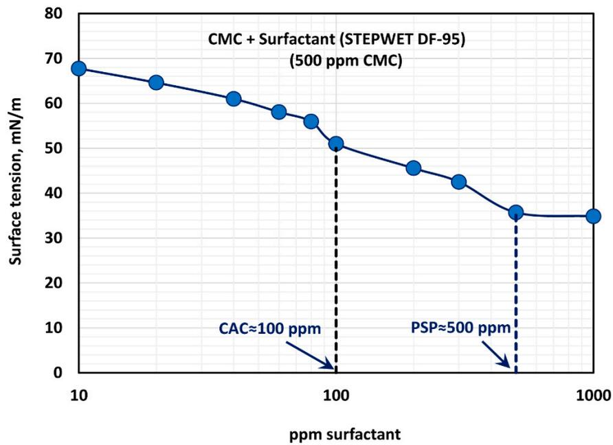
**Figure 7.** Variation of surface tension of surfactant-polymer solutions with the increase in surfactant concentration, at a fixed polymer concentration of 500 ppm.
