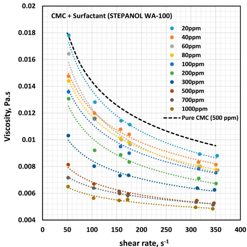
**Figure 8.** Effect of anionic surfactant (Stepanol WA-100) on the viscosity versus shear rate behavior of solutions of mixtures of anionic polymer, CMC, and anionic surfactant, Stepanol WA-100, at a fixed polymer concentration of 500 ppm.
