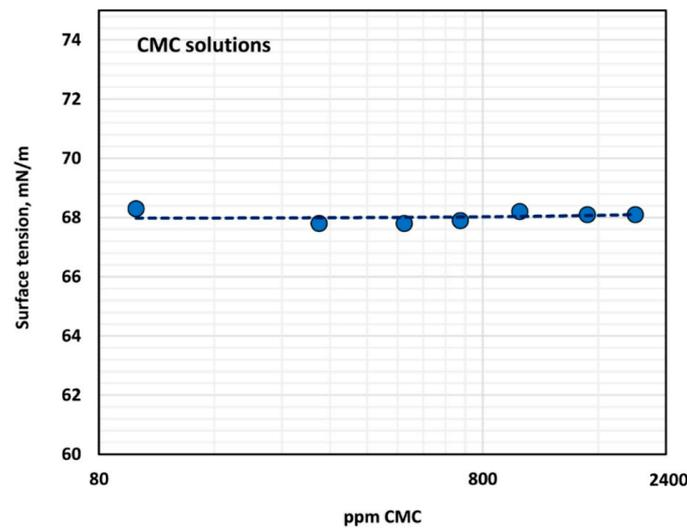
**Figure 4.** Variation of surface tension of polymer solution with the increase in polymer concentration.
