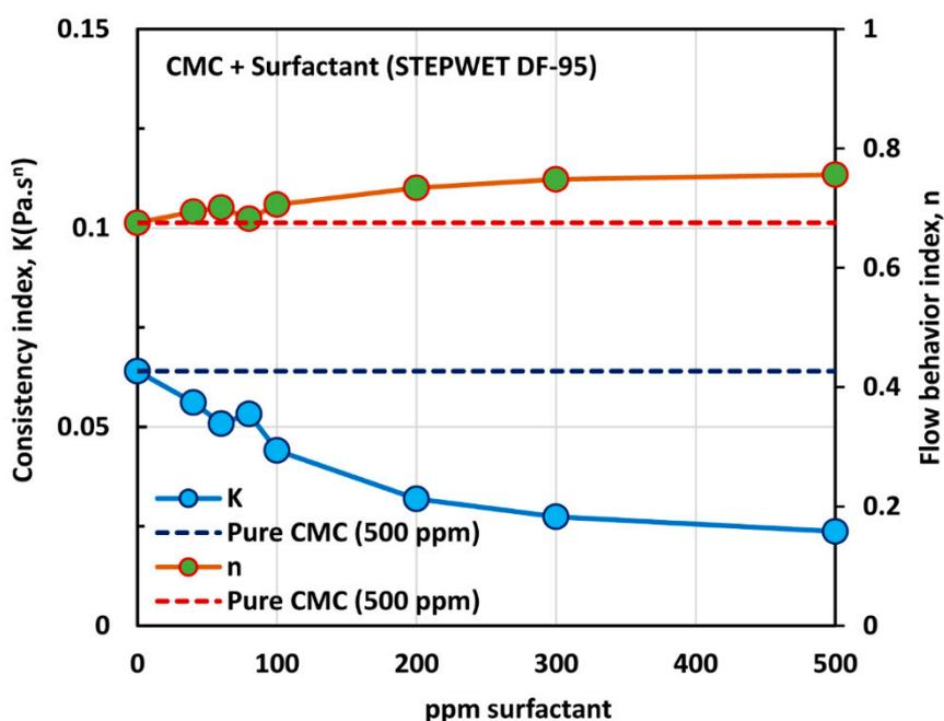
**Figure 6.** Variations of consistency index,  $K$ , and flow behavior index,  $n$ , for mixtures of anionic polymer, CMC, and anionic surfactant, Stepwet DF-95, with the increase in surfactant concentration, at a fixed polymer concentration of 500 ppm.
