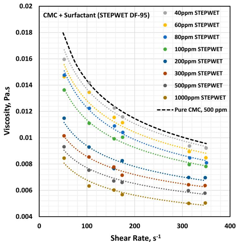
**Figure 5.** Effect of anionic surfactant (Stepwet DF-95) on the viscosity versus shear rate behavior of solutions of mixtures of the anionic polymer, CMC, and the anionic surfactant, Stepwet DF-95, at a fixed polymer concentration of 500 ppm.
