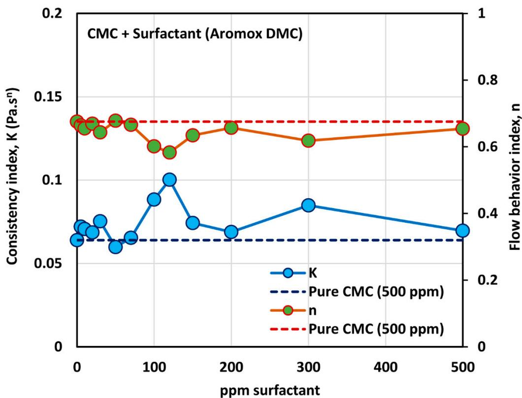
**Figure 15.** Variations of consistency index,  $K$ , and flow behavior index,  $n$ , for mixtures of anionic polymer, CMC, and non-ionic surfactant, Aromox DMC, with the increase in surfactant concentration, at a fixed polymer concentration of 500 ppm.
