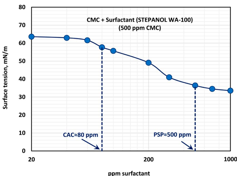
**Figure 10.** Variation of surface tension of surfactant-polymer solutions with the increase in surfactant (Stepanol WA-100) concentration, at a fixed polymer (CMC) concentration of 500 ppm.
