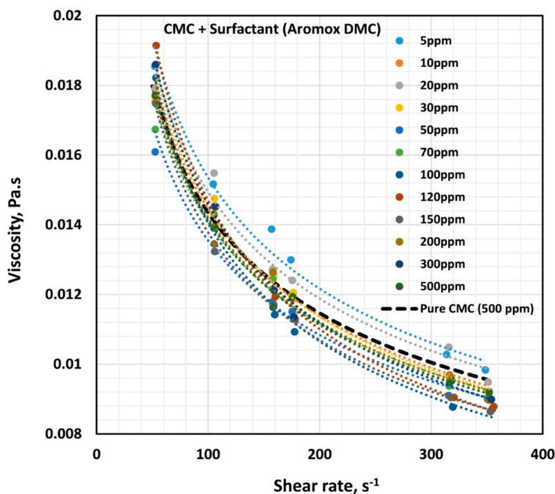
**Figure 14.** Effect of non-ionic surfactant (Aromox DMC) on the viscosity versus shear rate behavior of solutions of mixtures of the anionic polymer, CMC, and the non-ionic surfactant, Aromox DMC, at a fixed polymer concentration of 500 ppm.
