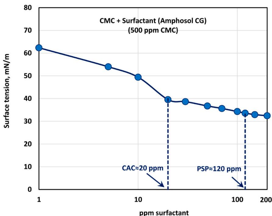
**Figure 19.** Variation of surface tension of surfactant-polymer solutions with the increase in surfactant (Amphosol CG) concentration, at a fixed polymer (CMC) concentration of 500 ppm.
