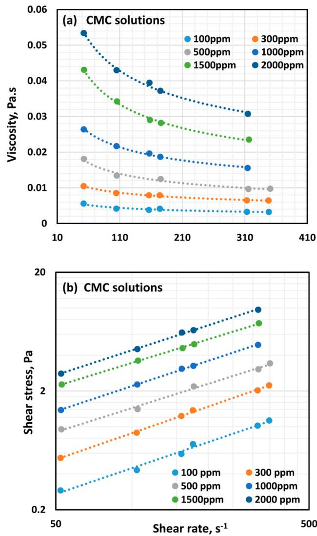
Figure 2. Flow curves for solutions of anionic polymer CMC at different polymer concentrations: (a) Viscosity versus shear rate and (b) Shear stress versus shear rate.
