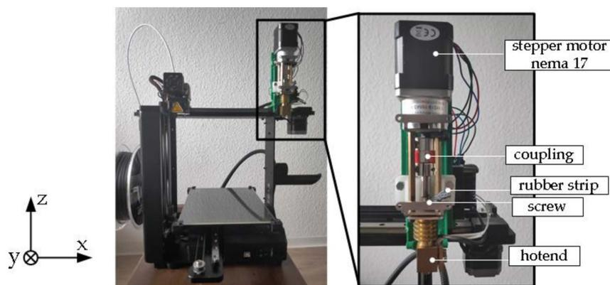
**Figure 1.** The MAKERGEAR M3-ID desktop 3D printer modified with a screw extruder.
