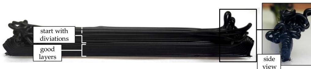
**Figure 5.** The printing result for stacking double strands. Seven to eight layers were laid well on top of each other until deviations occurred. The trigger of the deviations is probably caused by the reversal point, as the side view illustrates.
