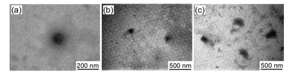
**Figure S1.** TEM images of PEG<sub>54</sub>-P(AA/VE6/ $\gamma$ TCP29)<sub>140</sub> at  $C_P$  = 0.10 g/L in PBS buffer of pH 7.4 (a), in acetate buffer of pH 5.2 just after preparation (b) and after 60 h (c).
