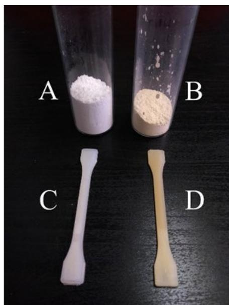
**Figure S1.** Visual comparison of HNTs (A) and HNT<sub>H</sub> (B) and their respective composites prepared via injection moulding: PA6<sub>melt</sub>\_HNTs\_4 (C) and PA6<sub>melt</sub>\_HNT<sub>H</sub>\_4 (D).
