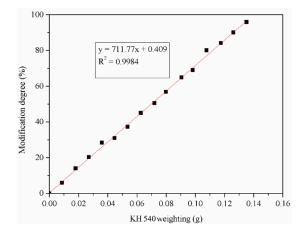
Figure S2. Effect of KH540 dosage on surface modification degree of nano-SiO2.
