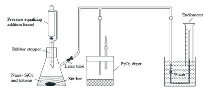
Figure S1. Flow-process diagram of CH<sub>3</sub>MgCl titration.
