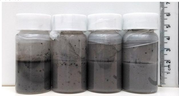
**Figure 4.** Toluene-in-water mixtures prepared from 2 wt% SiO<sub>2</sub> and 1 mg MWNTs with 0.2 M APTES and DTES. The emulsions occasionally show the presence of MWNT aggregates, as illustrated by black dots within the otherwise typically homogeneous, milky-grey mixtures. From left to right: o/w ratio = 10:90, 20:80, 30:70, 50:50.
