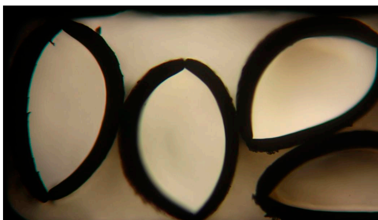
Figure S2. The cross-section of PEEK/PEI hollow fiber by optical microscope (100×).
