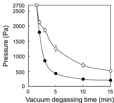
**Figure 1.** Relationship between pressure in the vacuum desiccator and vacuum degassing time. The sealed glass jar contained monomer solution (○) or did not contain monomer solution (●). Error bars indicate standard deviation.
