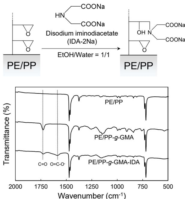
**Figure 5.** FTIR-ATR spectra of the PE/PP, PE/PP-g-GMA, and PE/PP-g-GMA-IDA fabrics.
