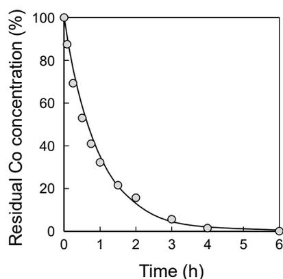
**Figure 6.** Co concentration (50 ppm) decay in water during the adsorption of Co(II) on PE/PP-g-GMA-IDA fabric.
