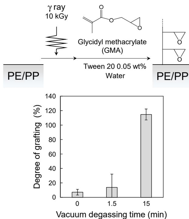
**Figure 2.** Relationship between degree of grafting and vacuum degassing time at 10 kGy. Error bars indicate standard deviation.
