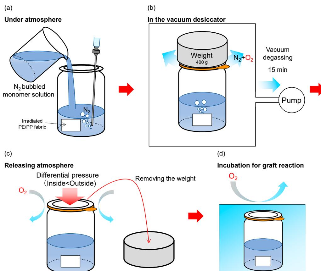
**Scheme 1.** Schematic image of a simplified radiation-induced emulsion graft polymerization (SREG).
