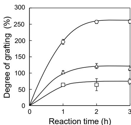
**Figure 4.** Graft polymerization using the SREG method at 20 (○), 10 (△), and 5 (□) kGy. Error bars indicate standard deviation.
