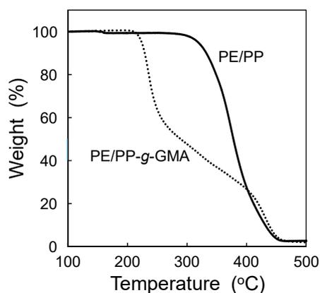
**Figure 3.** TGA curves for the PE/PP and PE/PP-g-GMA fabric under nitrogen.
