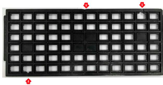
**Figure 8.** Short shot defects (without packing) for IC trays with under-filling.
