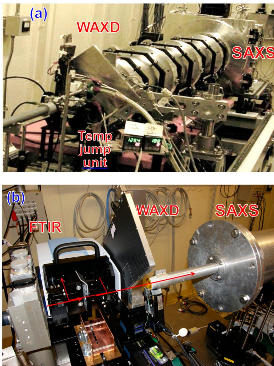
**Figure 1.** Simultaneous measurement systems in the synchrotron facilities. (a) WAXD and SAXS; (b) WAXD, SAXS, and FTIR spectra. In these two cases, the detectors were a flat panel (WAXD) and an image-intensifier-CCD (SAXS).
