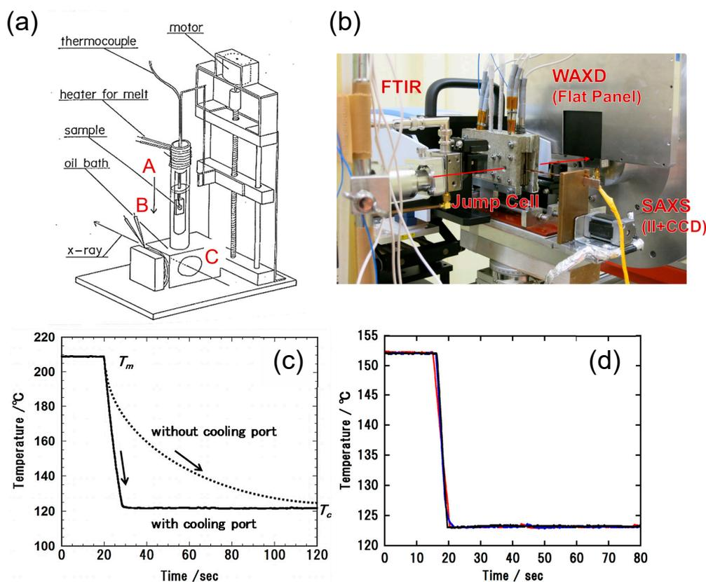
**Figure 2.** Temperature jump cells. (a) Manually operated system (the sample holder is moved vertically) and (b) computer-controlled system (the sample holder is moved horizontally from position (A) to (B) to (C)). (c) Temperature change in the sample in the temperature jump process with and without the cooling port at position (B) and (d) the reproducibility of the temperature change observed for the system (b).
