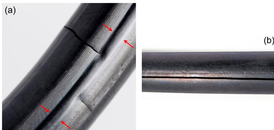
**Figure 12.** (a) Photo of seal N2 after failure and aging for 224 days at 150 °C. Red arrows indicate the recovered narrow rubbery region on the seal face. (b) Photo of EPDM O-ring aged in the uncompressed state for 1 year at 150 °C with a deep circumferential crack.
