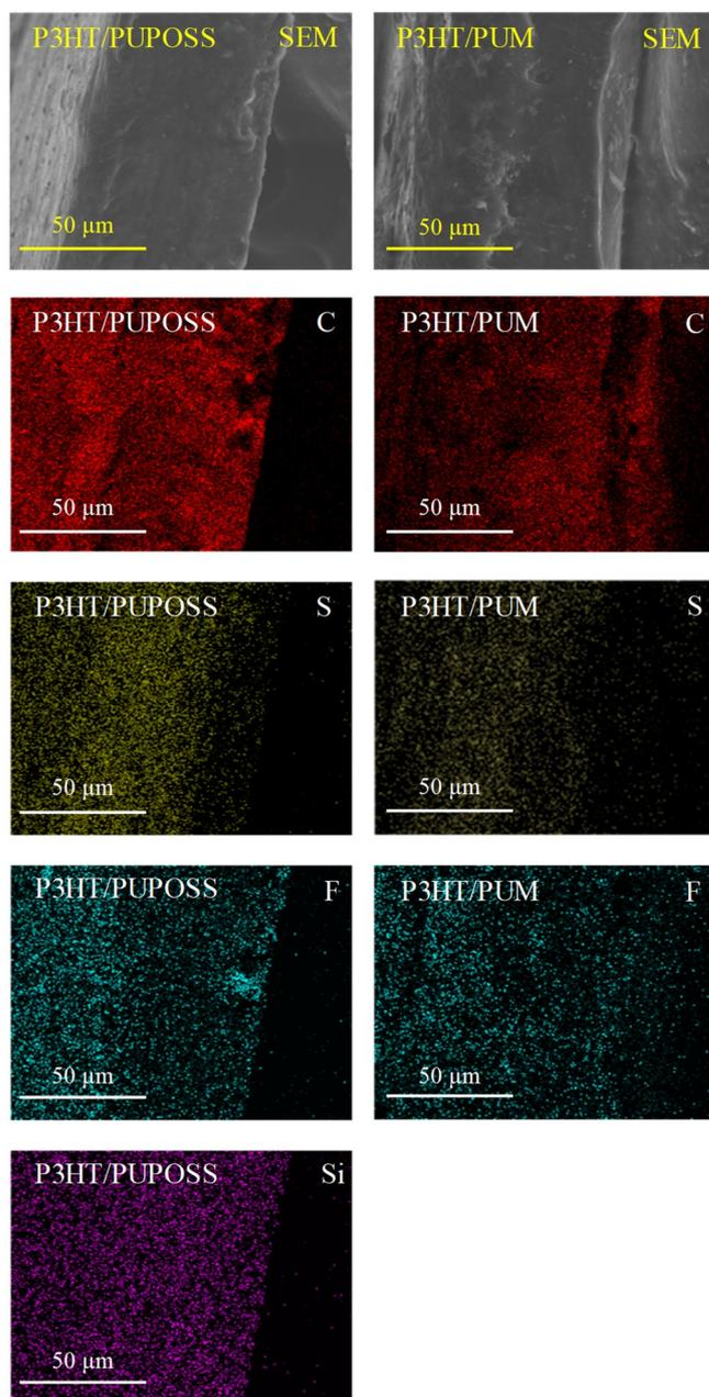
**Figure S10.** SEM images and elemental mapping of the cross section of hybrid films. The amount of doped P3HT loaded in all films is 20 wt%. Right side of the images is the interface of hybrid film/air.
