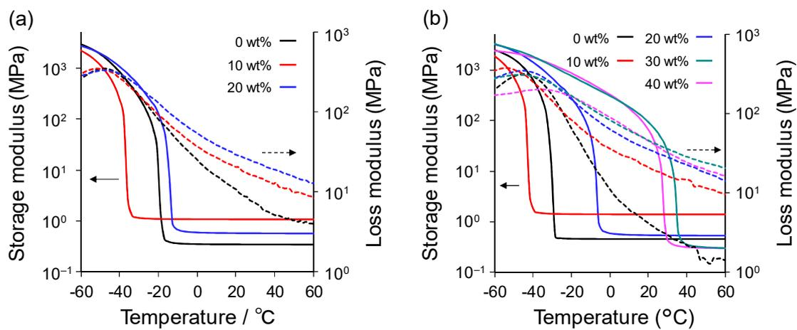
**Figure S11.** Storage and loss moduli of (a) P3HT/PUPOSS and (b) P3HT/PUM at each amount of loaded doped P3HT.
