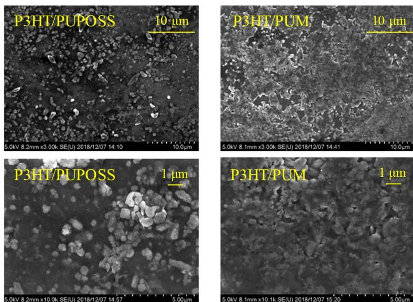
**Figure S9.** SEM images of the surface of hybrid films (interface of hybrid film/PFA dish). The amount of doped P3HT loaded in all films is 20 wt%.
