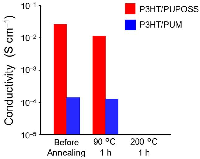
**Figure S13.** In-plane electrical conductivity of P3HT/PUPOSS and P3HT/PUM loading 20 wt% of P3HT before and after thermal annealing.
