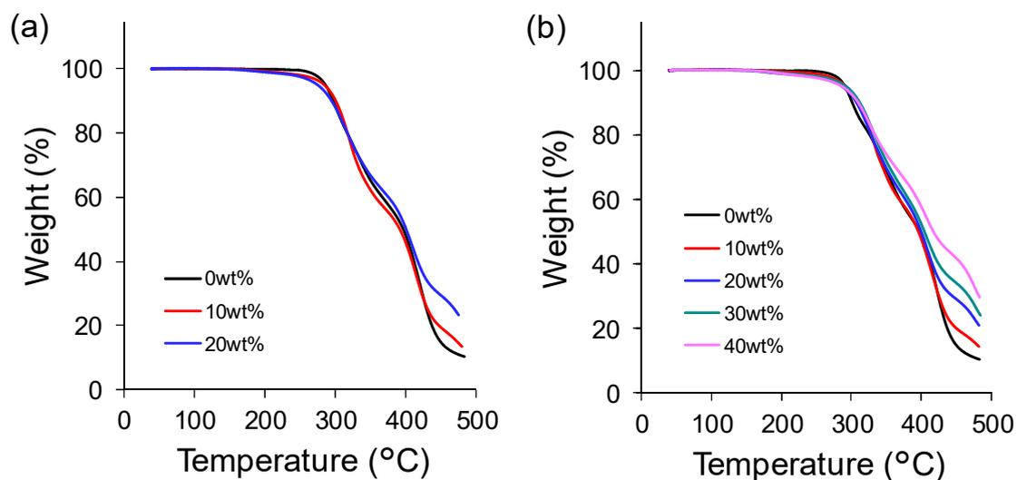
**Figure S12.** TGA curves of (a) P3HT/PUPOSS and (b) P3HT/PUM at each amount of loaded doped P3HT.
