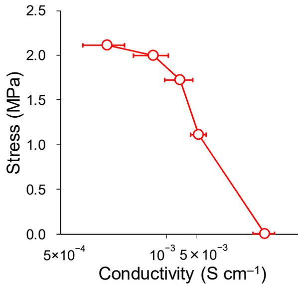
**Figure S14.** The relationship between conductivity and applied mechanical forces of P3HT/PUPOSS loaded 20 wt% of doped P3HT.
