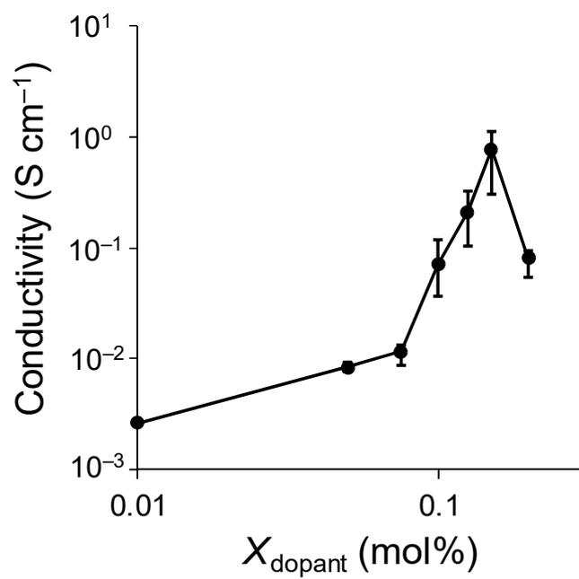
Figure S7. In-plane conductivity of F4-TCNQ doped P3HT films.
