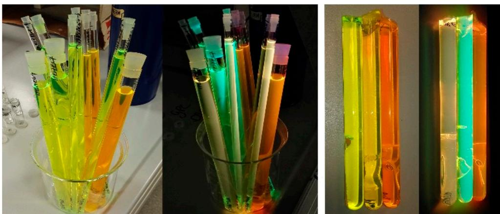
**Figure 2.** Photographs of the solutions before (left) and after (right) polymerization under environmental lighting and UV excitation.
