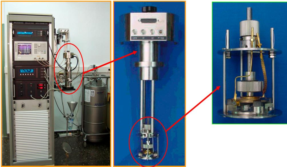
**Figure S6.** Schematic illustration of the Novocontrol Concept 80.
