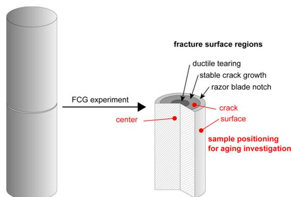
**Figure 2.** Schematic of the CRB specimen (left) before and (right) after fatigue crack growth (FCG) experiments indicating the three sample positions (i.e., center, surface, and crack) for the investigation of the corresponding local aging states.
