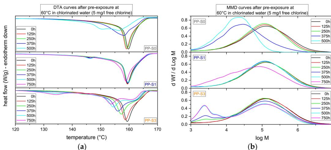
**Figure 3.** (a) Differential thermal analysis (DTA) curves indicating the melting peaks in the second heating step and (b) molar mass distribution (MMD) curves for various exposure times of micro-sized specimens to chlorinated water (5 mg/L free chlorine) at 60 °C for the three polypropylene (PP) grades.
