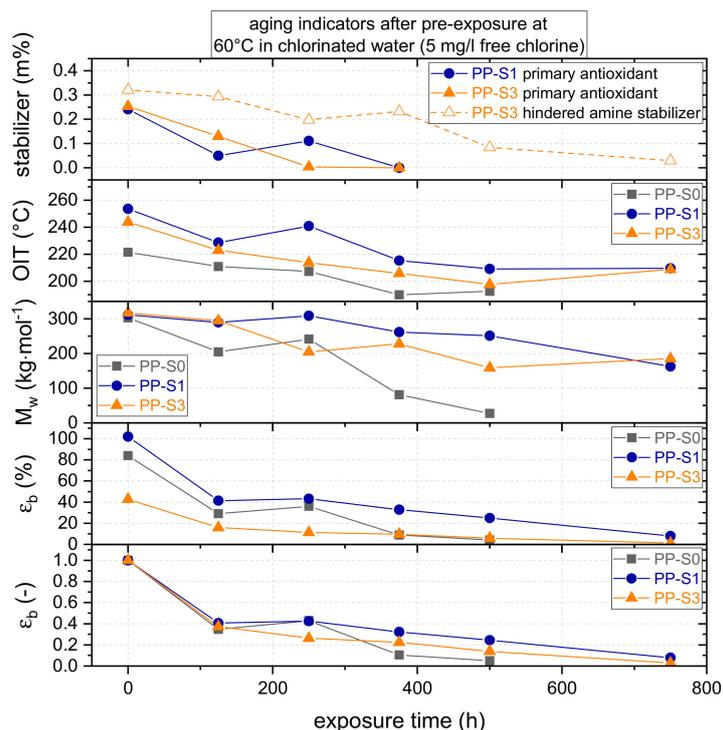
**Figure 4.** Stabilizer content (primary antioxidants and hindered amine stabilizer), dynamic oxidation induction temperature (OIT), mean weight average molar mass ( $M_w$ ), strain at break ( $\epsilon_b$ ), and normalized strain at break as a function of exposure time of micro-sized specimens for the three PP grades.
