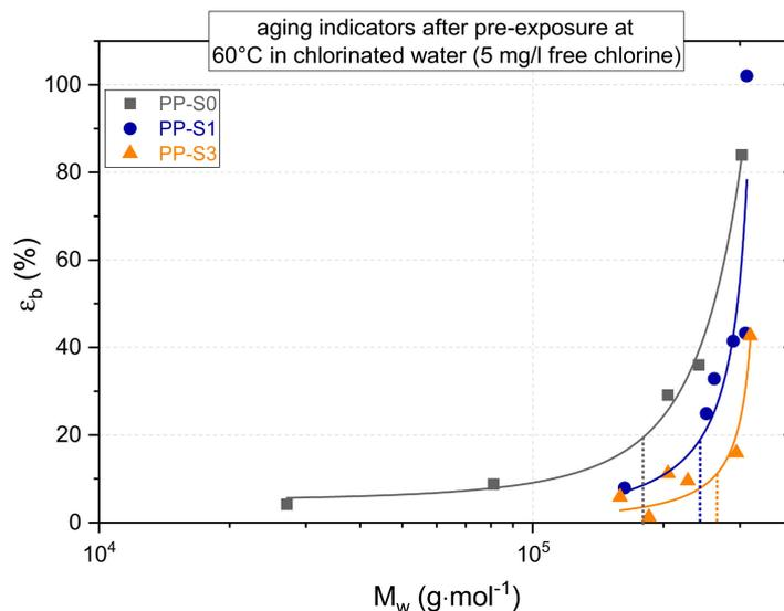
**Figure 7.** Dependence of strain at break values ( $\epsilon_b$ ) of the three aged PP grades on the mean molar mass ( $M_w$ ) of these materials in the aged state with indications on the vertex (dotted line) of the fit curvature representing the characteristic embrittlement mean molar mass of the materials (PP-S0: 180 kg/mol), PP-S1: 243 kg/mol, PP-S3: 265 kg/mol).
