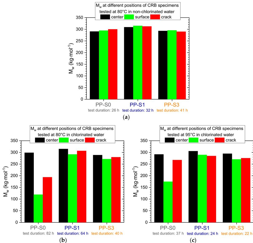
**Figure 6.** Mean weight average molar masses ( $M_w$ ) of samples taken from three different positions in CRB specimens of PP-S0, PP-S1, and PP-S3, which were tested under superimposed mechanical-environmental conditions. The fatigue crack growth tests were performed at (a) 80 °C in non-chlorinated water (0 mg/L free chlorine); (b) 80 °C in chlorinated water (5 mg/L free chlorine); and (c) 95 °C in chlorinated water (5 mg/L free chlorine). The total FCG test duration is also indicated.
