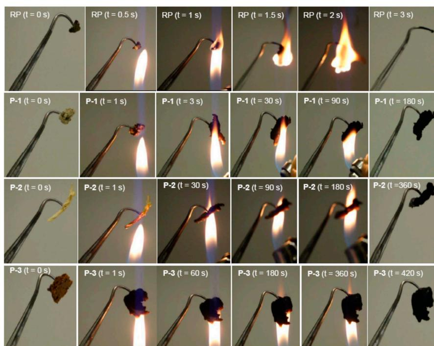
**Figure 13.** Photographs taken during direct flaming/combustion of a reference polymer (**RP**; top row) and ionic polymers (**P-1**, **P-2**, and **P-3**) (bottom three rows).
