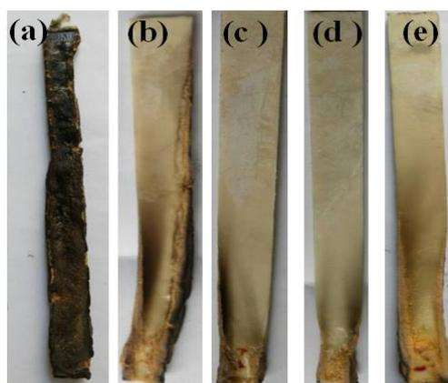
**Figure 6.** Digital photographs of PLA/GNR and PLA/GNR/SiAHP composites after UL-94 vertical burning tests. (a) PLA/GNR/16wt%AHP; (b) PLA/GNR/16wt%SiAHP; (c) PLA/GNR/18wt%SiAHP; (d) PLA/GNR/20wt%AHP; (e) PLA/GNR/20wt%SiAHP.
