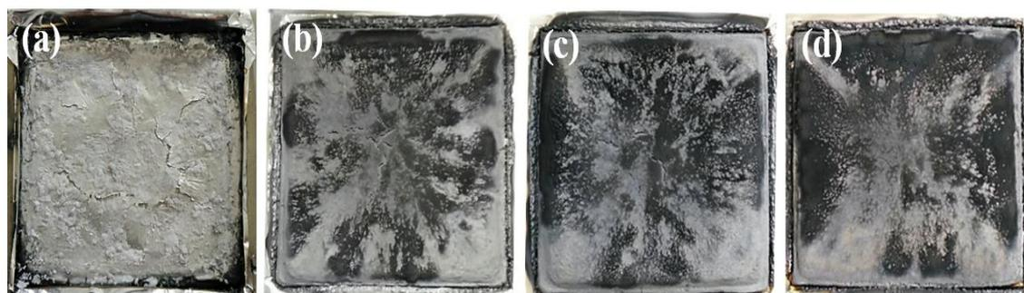
**Figure 10.** Digital photos of char residues for PLA/GNR TPV (a); PLA/GNR/16wt%SiAHP (b); PLA/GNR/18wt%SiAHP (c); PLA/GNR/20wt%SiAHP (d) after the cone calorimeter test.
