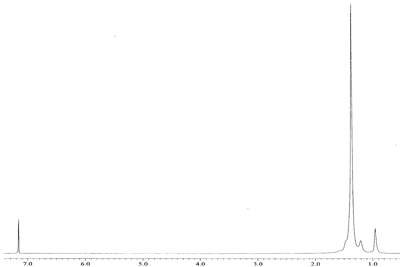
Figure S29. ^1\text{H} NMR spectrum of polymer (entry 3 in Table 1).
