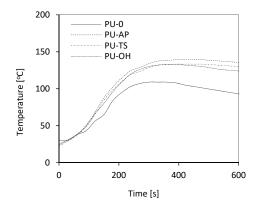
Figure 6. Temperature of reaction mixture in PU formulations.
