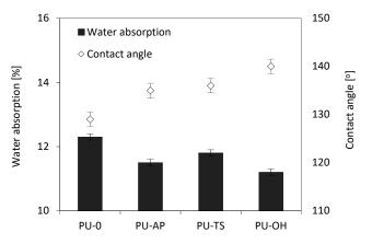
Figure 17. Effect of contact angle on water absorption of RPUFs modified with POSS.
