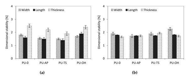
**Figure 16.** Dimensional stability of RPUFs modified with AP-POSS, TS-POSS and OH-POSS after exposure at 70  $^{\circ}$ C (**a**) and -20  $^{\circ}$ C (**b**).
