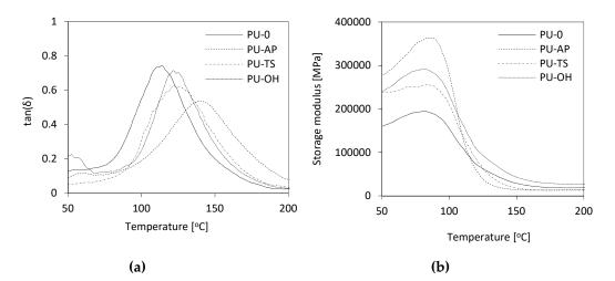
**Figure 14.** (a) tanδ and (b) storage modulus as a function of temperature plotted for RPUFs.
