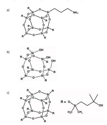
Figure 1. Chemical structure of (a) AP-POSS, (b) TS-POSS and (c) OH-POSS.
