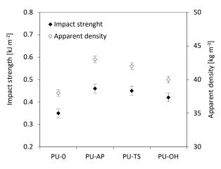
Figure 13. Effect of apparent density on the impact strength of RPUFs.
