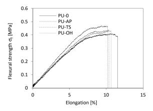
Figure 12. Flexural stress-elongation curves of RPUFs.
