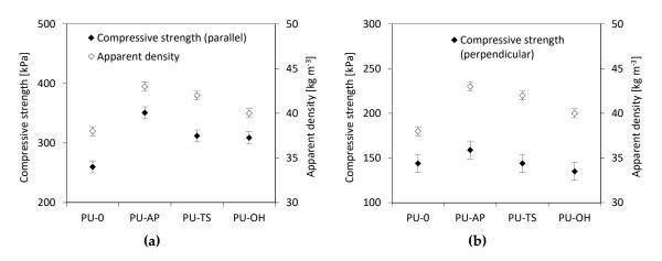
**Figure 10.** Effect of apparent density on compressive strength of RPUFs of RPUFs measured (**a**) parallel and (**b**) perpendicular to the foam rise direction.
