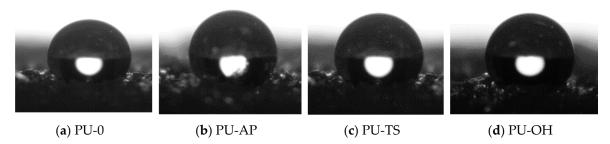
Figure 18. The contact angle of the surface of the (a) PU-0, (b) PU-AP, (c) PU-TS, (d) PU-OH.
