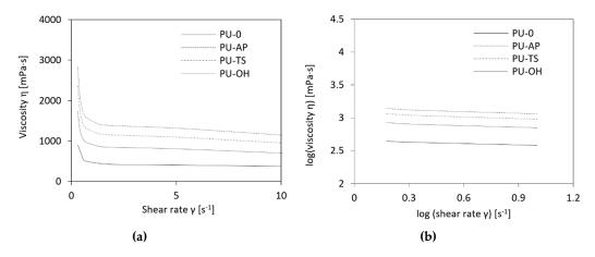
**Figure 5.** (a) Viscosity as a function of shear rate and (b) log-log plot of the viscosity vs. the shear rate for polyol premixes.
