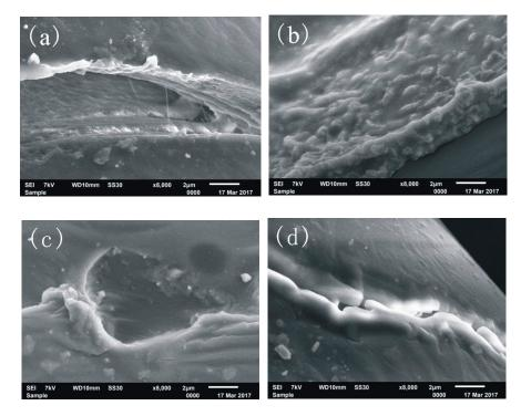
Figure 6. Four structure defects of sutures: (a) peeling, (b) swelling, (c) corrosion hole, (d) ditch.
