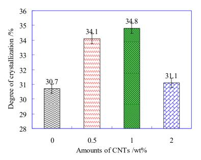
Figure 4. Degree of crystallization of PLA fiber with different contents of CNTs.
