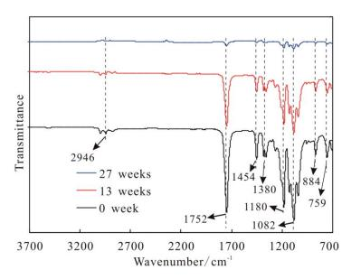
**Figure 11.** The fourier transform infrared spectra (FTIR) of 1 wt% CNTs/PLA sutures at different degradation time points.
