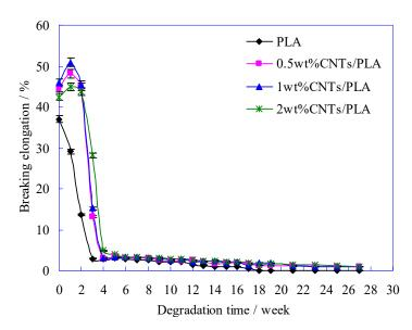
Figure 9. The variation of breaking elongation of PLA-base sutures with degradation time.
