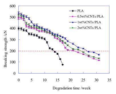
Figure 7. Breaking strength of pure PLA suture and CNTs/PLA sutures during degradation.
