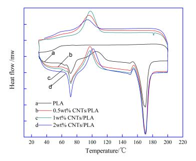
Figure 3. DSC curves of PLA sutures with different contents of CNTs.
