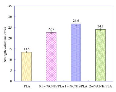
Figure 8. The strength valid time of pure PLA suture and CNTs/PLA sutures.
