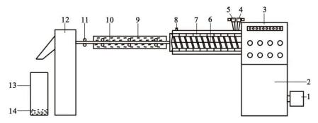
**Figure 1.** Diagrammatic sketch of the preparing machine for making carbon nanotubes (CNTs)/ Poly(lactic acid) (PLA) master batches. 1— main motor, 2—transmission case, 3— parameter adjustment controller, 4— main feed throat, 5— side feed throat, 6—twin screws, 7— ten heating zones, 8—vacuum pump, 9—cooling water bath, 10—CNT/PLA composite ribbon, 11—pulling rollers, 12—dicing cutter, 13—storage vat, and 14—CNTs/PLA master batches.
