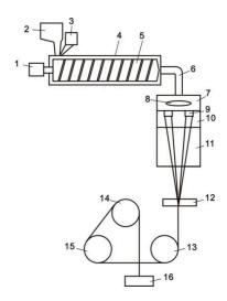
**Figure 2.** Sketch diagram of melt spinning of CNTs/PLA composite filaments. 1—screw machine, 2—main feed throat, 3—side feed throat, 4—four heating zones, 5—single screw, 6—elbow pipe, 7—spinning box, 8—metering pump, 9—spinning pack, 10—annealing device, 11—cooling device, 12—oil roller, 13—the first hot roller, 14—the second hot roller, 15—the third hot roller, and 16—winding device.
