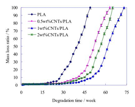
Figure 10. Change of mass loss ratio during degradation weeks.
