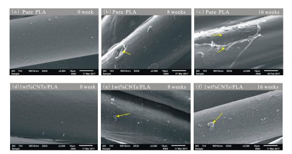
**Figure 5.** SEM images of surface morphology of sutures at different degradation time points: (**a**) pure PLA suture degraded for 0 week, (**b**) pure PLA suture degraded for 8 weeks, (**c**) pure PLA suture degraded for 16 weeks; (**d**) 1 wt% CNTs/PLA suture degraded for 0 week, (**e**) 1 wt% CNTs/PLA suture degraded for 16 weeks.
